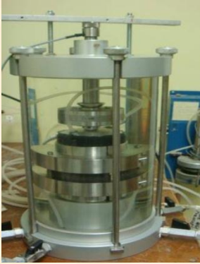
The new permeameter for swelling clays: "Porous rigid wall flexible wall permeameter"
