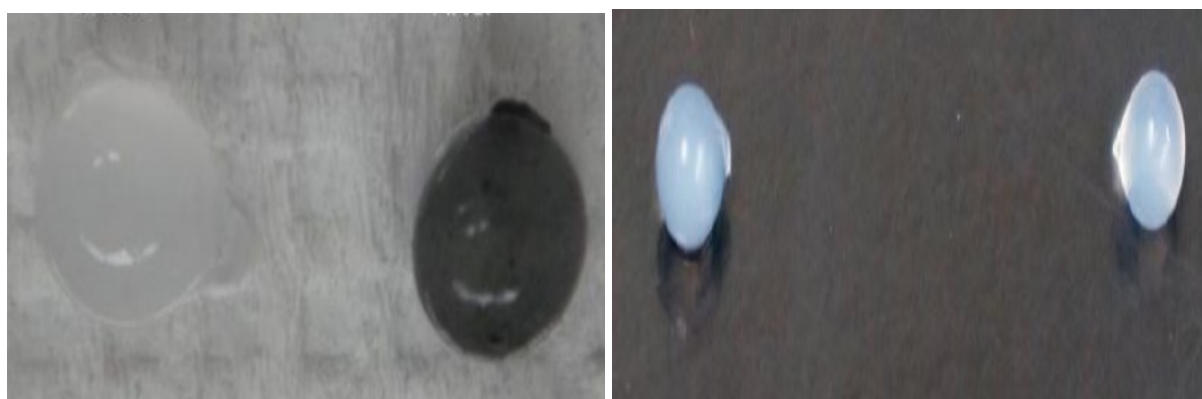
Figure 4-4: Entrapment beads before and after exposure to 500 \mu\text{g}/\text{ml} of long SWCNTs. (A) PVA beads, and (B) alginate beads.
