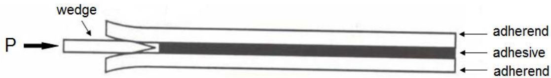
Fig. 2.16. Schematic representation of ASTM D 3762 wedge test
