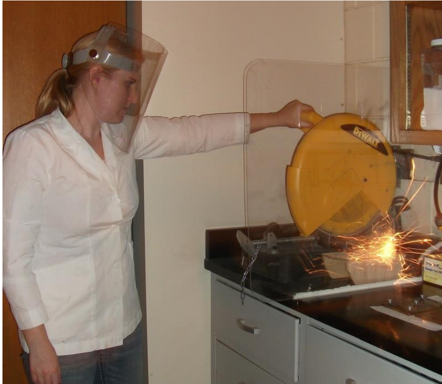
Figure 4.3. Preparing ice-cemented samples for processing. The ends of ice-cemented sample drill bits, and the small unconsolidated conduit samples were cut off using a masonry chop saw equipped with a diamond edged abrasive blade.
