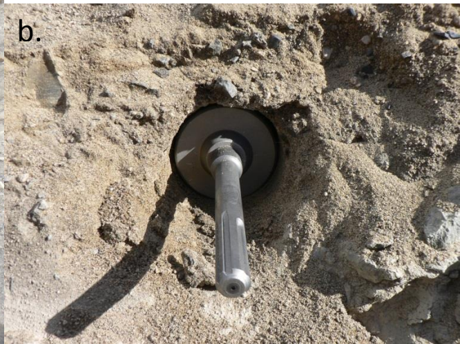
Figure 4.2. Collection of Ice-cemented sediments. a.) Ice-cemented sediments were collected using a rotary hammer drill with a concrete coring bit. The ice-cemented samples were collected and shipped still frozen to the laboratory. b.) The coring bit in the pit wall. Photographs courtesy of Adam Lewis.
