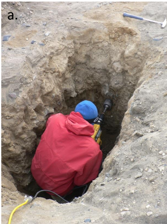
Figure 4.2. Collection of Ice-cemented sediments. a.) Ice-cemented sediments were collected using a rotary hammer drill with a concrete coring bit. The ice-cemented samples were collected and shipped still frozen to the laboratory. b.) The coring bit in the pit wall. Photographs courtesy of Adam Lewis.
