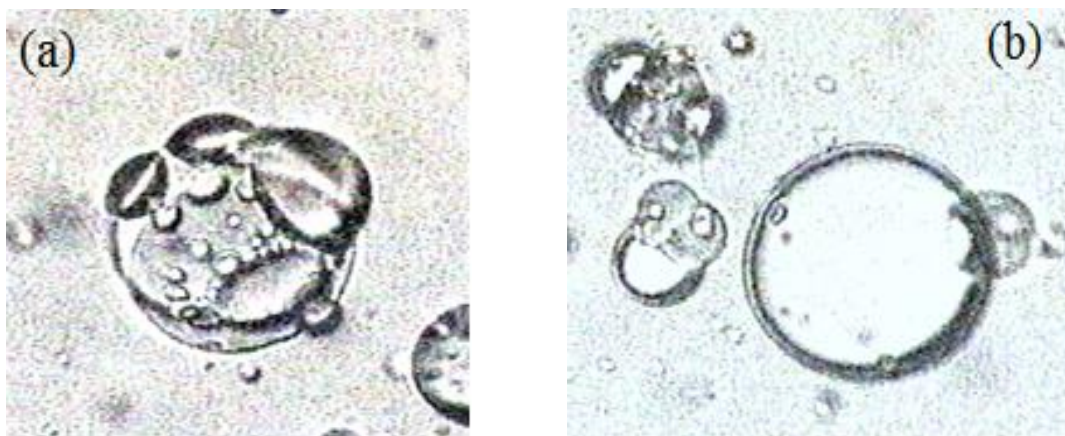
Figure 3.3. Formation of core-shell type capsules synthesized using internal phase separation observed using optical microscope at 20X (a) emulsion droplet showing internal phase separation with nucleation of polymer rich phases (b) emulsion droplet with a distinct polymer shell formed around water.
