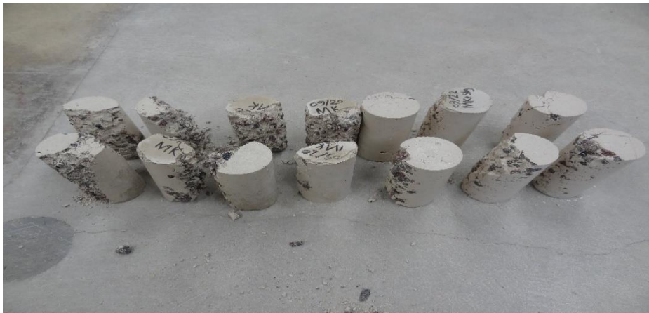
Figure 21. Effect of 30 cycles of freeze-thaw on cylindrical geopolymer concrete specimens
