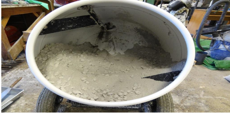
Figure 16. Mixer used for manufacturing geopolymer concrete
