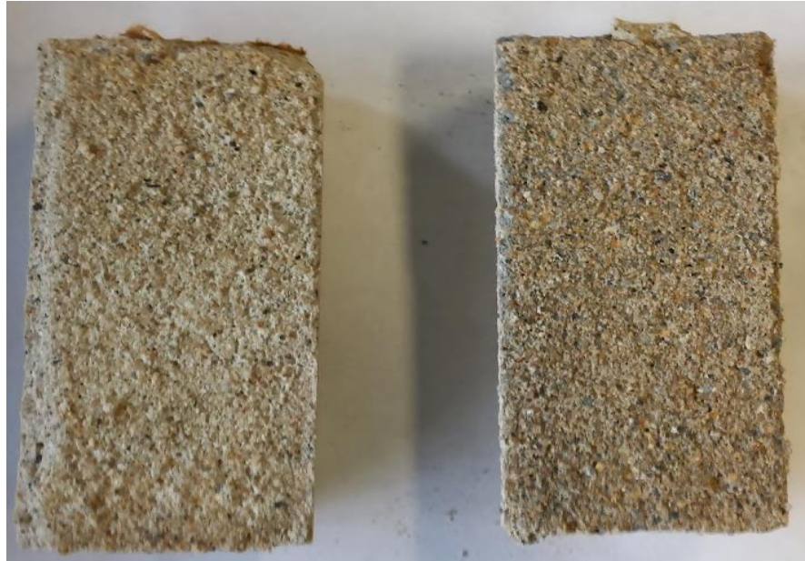
Figure 6. Failure mode between metakaolin-based geopolymer mortar and conventional concrete
