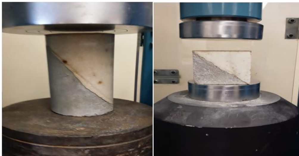
Figure 8. Slant shear test with line interface of 30° and 45°
