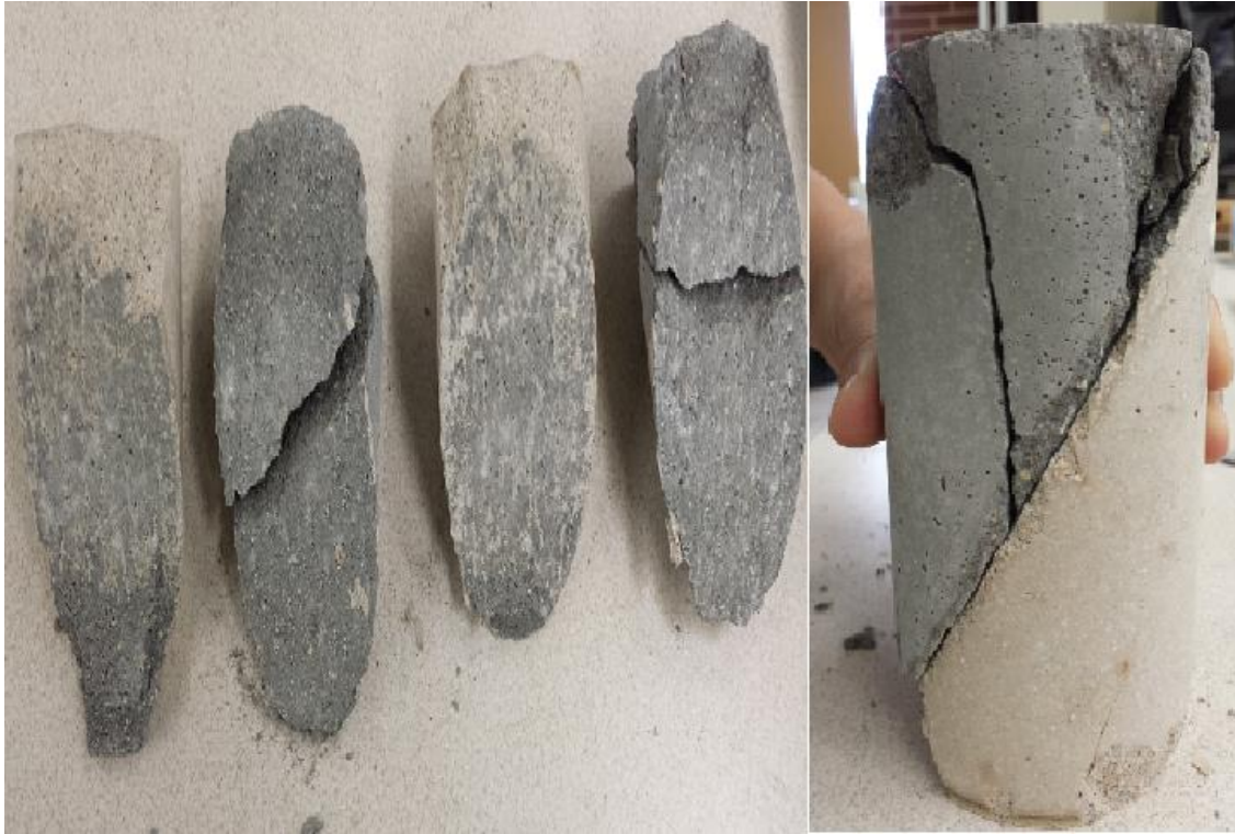
Figure 9. Failure mode of slant shear test with line interface at 30^\circ between metakaolin-based geopolymer mortar and conventional mortar
