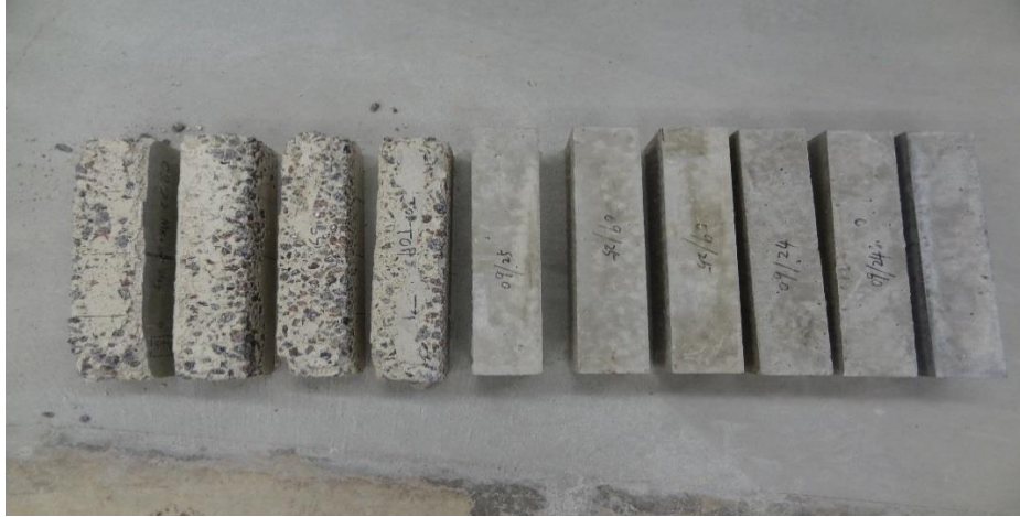
Figure 20. Surface of geopolymer concrete specimens after 30 cycles of freeze-thaw
