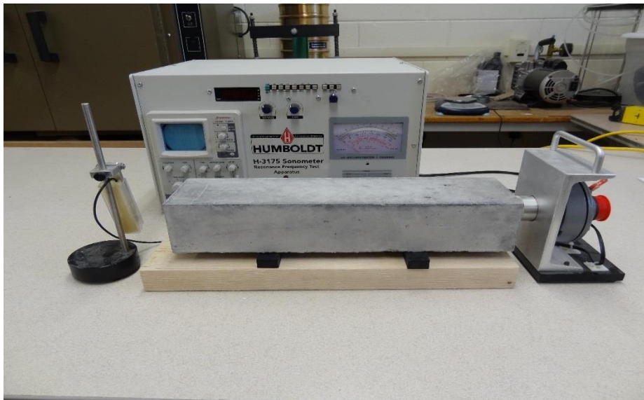
Figure 19. Sonometer used in determining dynamic modulus of freeze-thaw test specimens
