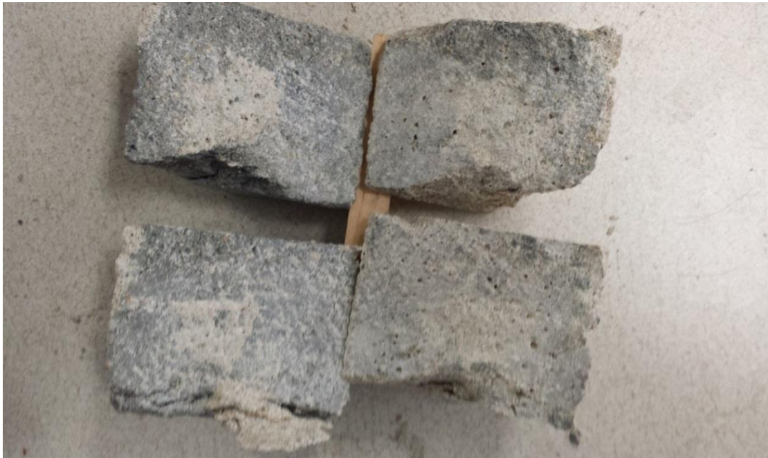
Figure 10. Failure mode of slant shear test with line interface at 45^\circ between metakaolin-based geopolymer mortar and conventional mortar
