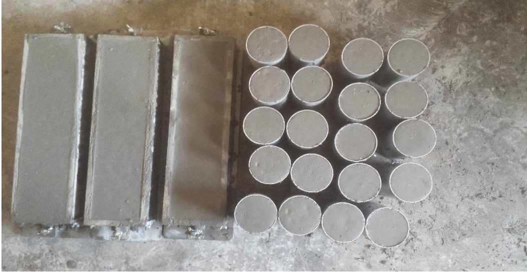
Figure 17. Fresh geopolymer concrete specimens (Mix-5)
