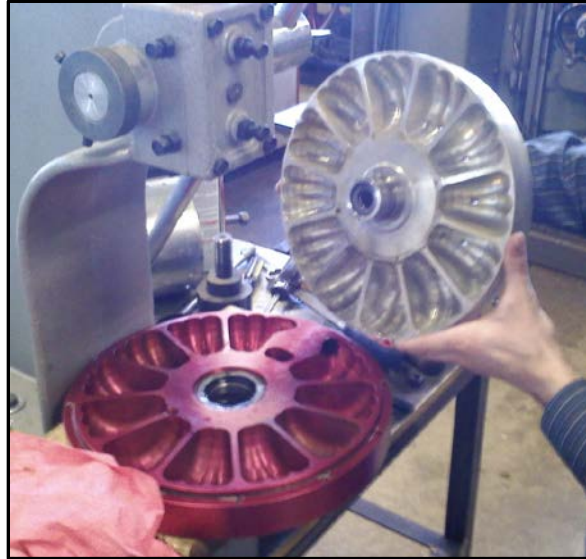
Figure 4. Inside View of the Water Brake Dynamometer
