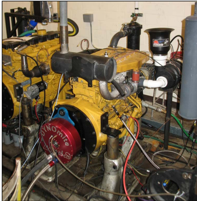
Figure 1. 4000 cc CAT Research Engine Setup in Lab
