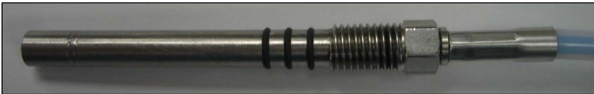
Figure 8. Insertion End of the In-Cylinder Pressure Sensor
