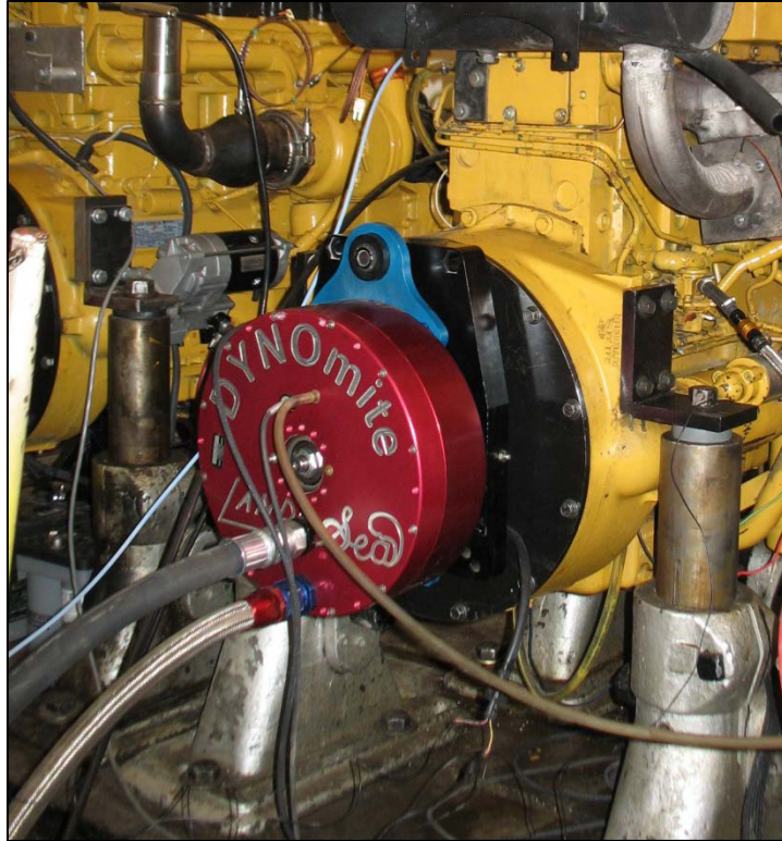
Figure 5. Dynamometer Mounted on CAT Engine
