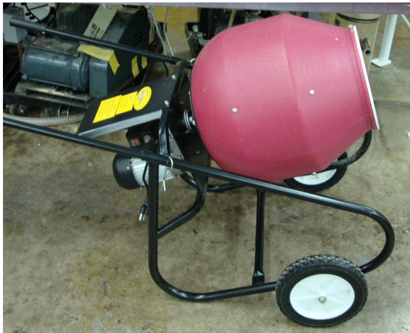
Figure 10 – Cement Mixer used to Agitate DDGS and Wood Fiber
