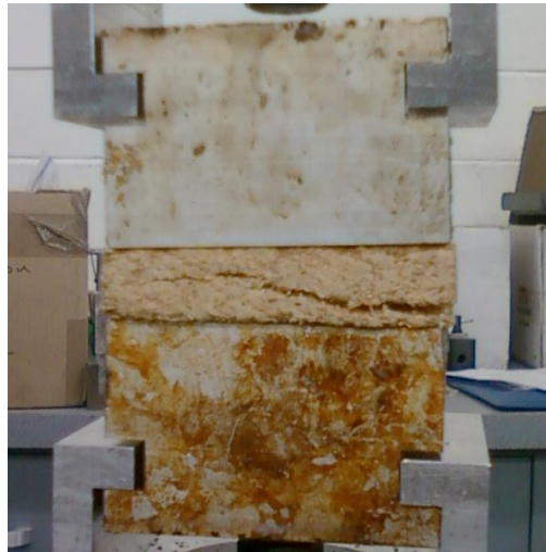
Figure 15 – Internal Bond Test Fixture and Loading Blocks
