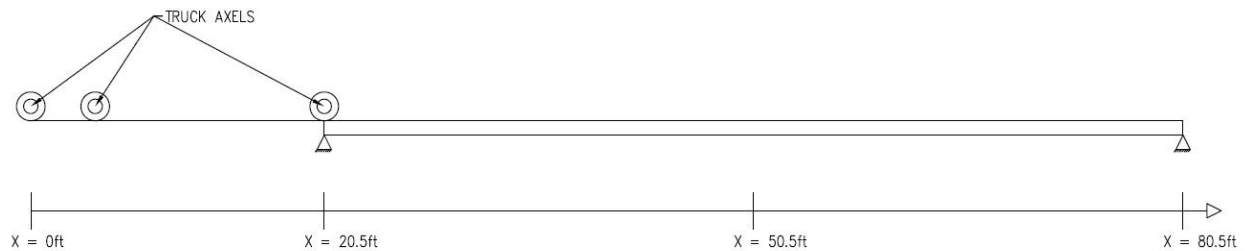
Figure 2.19. Relative bridge position
