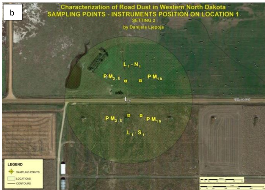
Figure 8. Maps of instrument locations at Location 1. a. Instrument positions at location 1(setting 1); b. Instrument positions at location 1 (setting 2).
