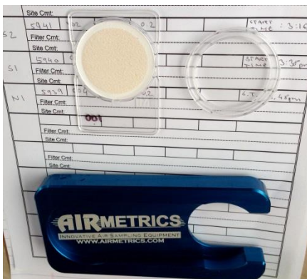
Figure 14. Cassette separator and filter.
