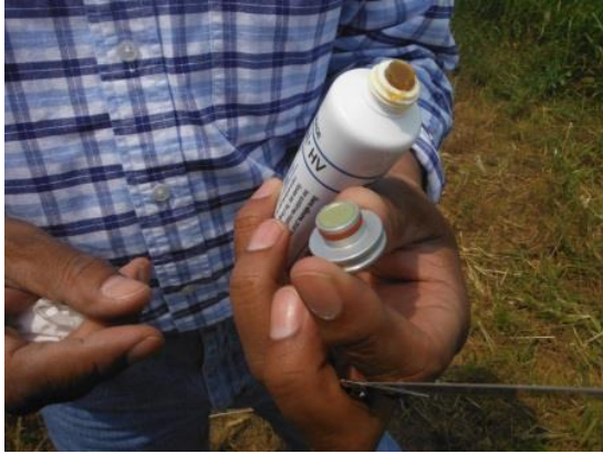
Figure 13. Applying grease to the EMT impactor. Sampling Site 1.
