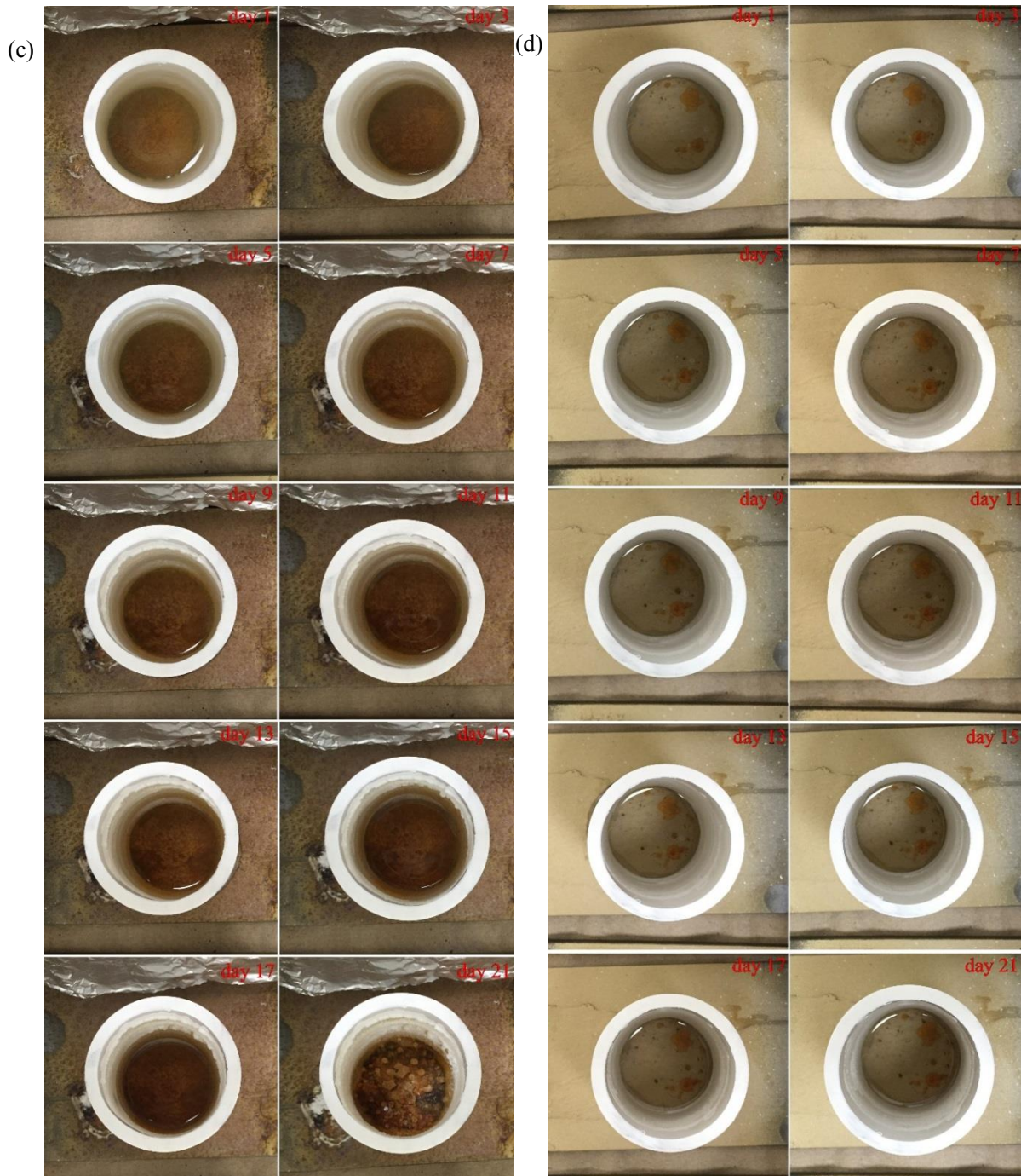
Figure 30. Corrosion visual inspection for Sample (a) #1, (b) #2, (c) #3, and (d) #4 (continued)
