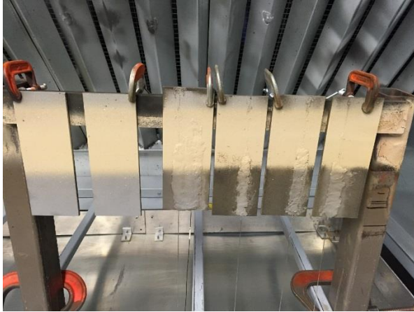
Figure 24. Thermal Spraying Coated Samples
