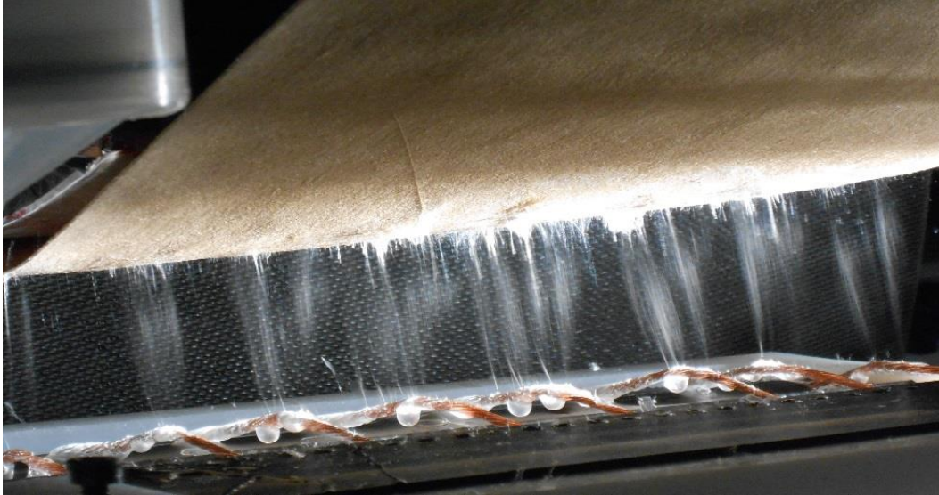
Figure 6-7: Mass production of soy based nanofibers using needleless electrospinning
