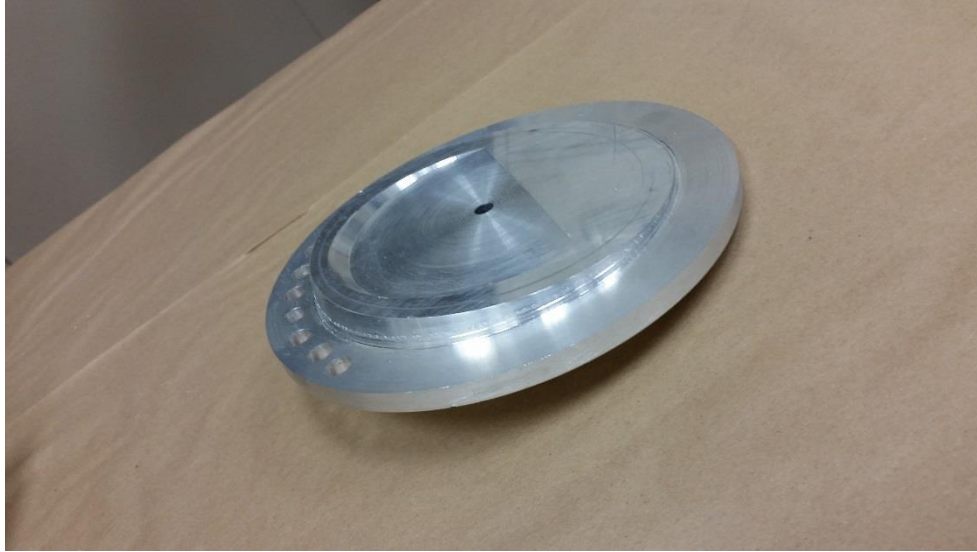
Figure 6-4: Initially designed cam, fabricated from steel
