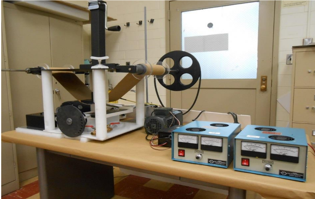
Figure 6-9: Image of completed needleless electrospinning machine
