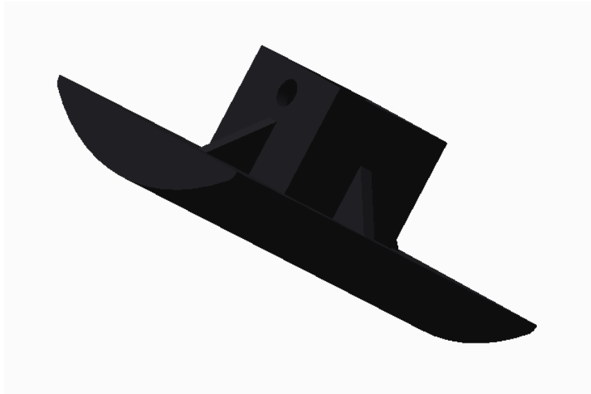
Figure 6-3: Collecting plate used on needleless electrospinning machine
