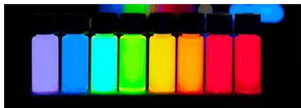
Figure 1.3. Quantum dots of increasing size will emit, when properly excited, with increasingly lower energy photons due to the quantum confinement effect. Quantum dots above were produced by PlasmaChem and are reprinted under the Creative Commons Attribution-Share Alike 3.0 Unported License.
