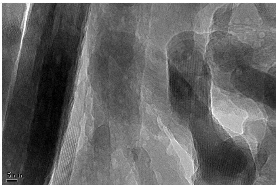
Figure F.38. TEM image of \beta -TCP showing lattice structure (x200,000 original magnification).
