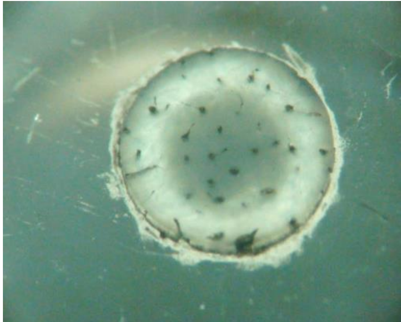
Figure C.13. A 70 micron thick 3 mm disc after dimpling and polishing ( <20 \mu\text{m} in depth) using the Gatan dimple grinder.
