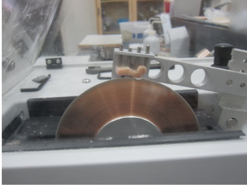
Figure C.2. Buehler low-speed saw equipped with diamond blade used for cutting 500-700 \mu\text{m} longitudinal and transverse sections from the stock bone samples.
