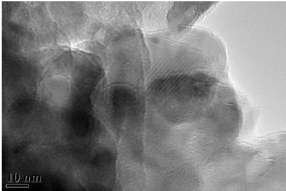
Figure F.34. TEM image of in-situ HAPclay showing lattice structure (x200,000 original magnification).
