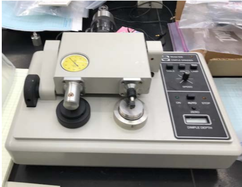
Figure C.11. Gatan dimple grinder model 656.
