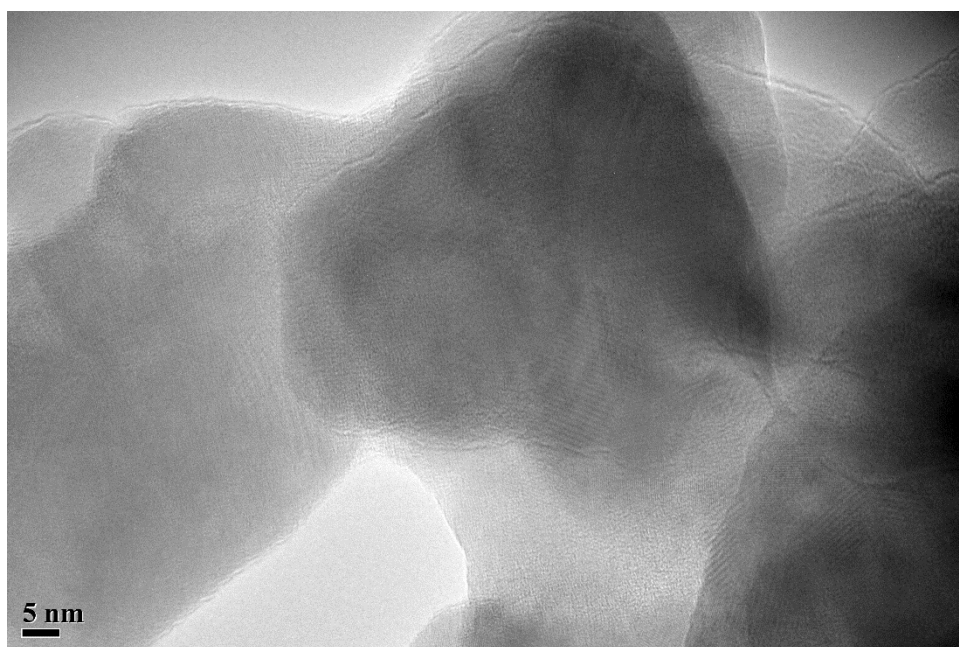
Figure F.24. TEM image of HAP showing lattice structure (x200,000 original magnification).
