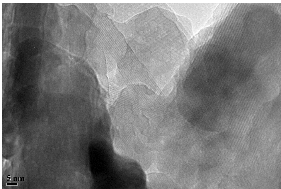
Figure F.44. TEM image of \beta -TCP showing lattice structure (x200,000 original magnification).
