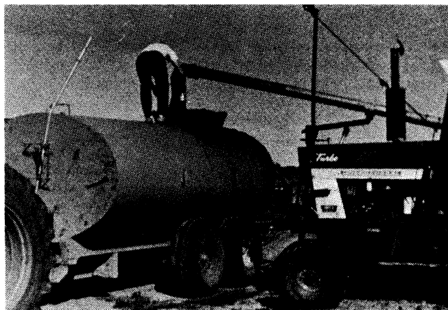
Figure 5. Sampling of liquid manure was done after tank contents were agitated and about one-third of the storage volume had been pumped and hauled.
