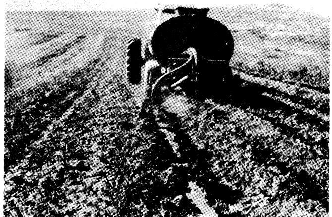
Figure 4. Plowing down immediately following broadcasting or knifing-in liquid manure minimizes odor problems and nutrient loss when field spreading. Application rate is limited, however, and power requirement is increased. Godwin, et al (1985) reported winged applicator tines reduced draft 50 percent and improved application efficiency compared to narrow tines.
