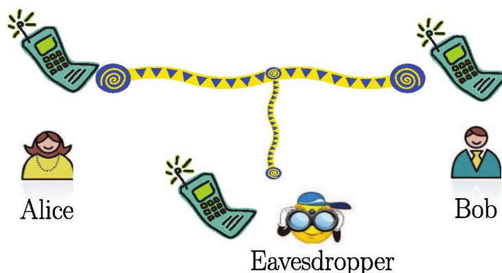
Figure 5.1. A Practical Wiretap Channel.
