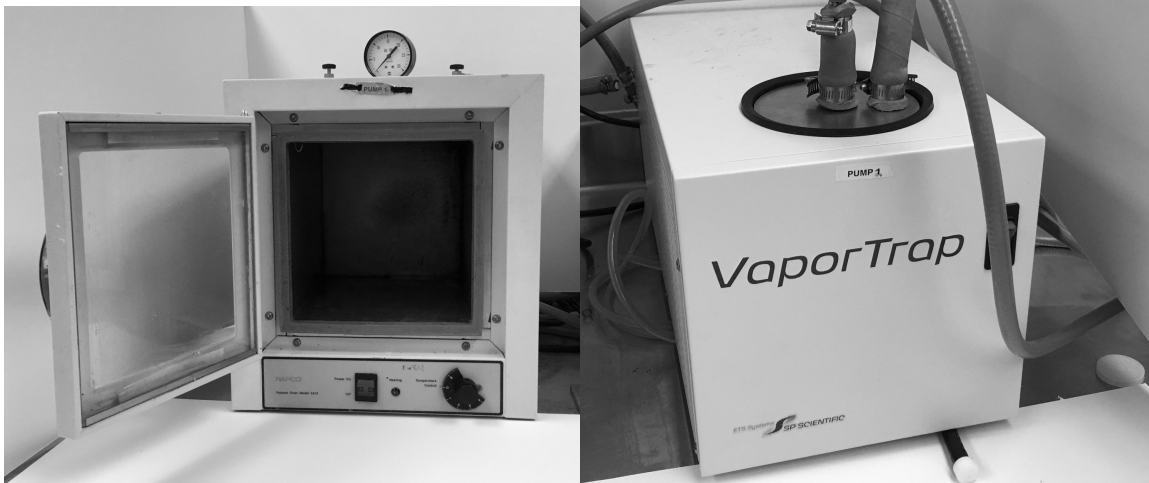
Figure 3: The vacuum oven acted as a vacuum reservoir for the VFFS and to remove solvents from the finished film (left). The Vapor Trap kept gaseous water from entering the vacuum pump (right).
