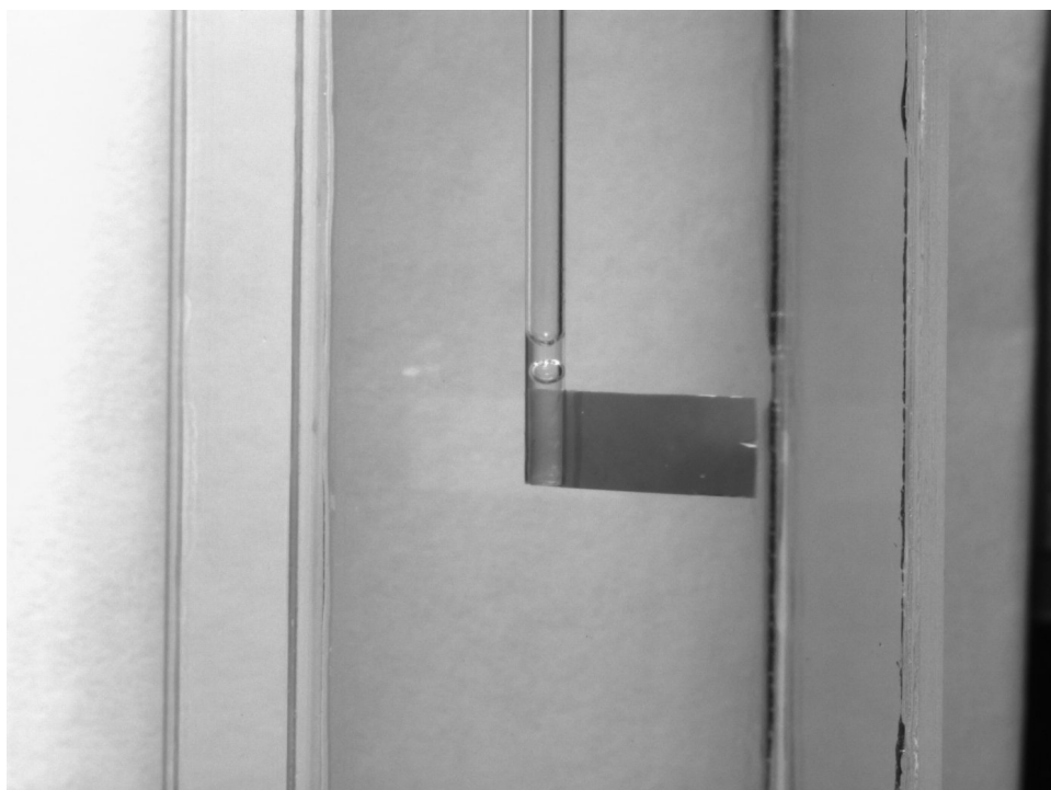
Figure 15: A nanofilm on filter paper attached to the inside of a glass tube
