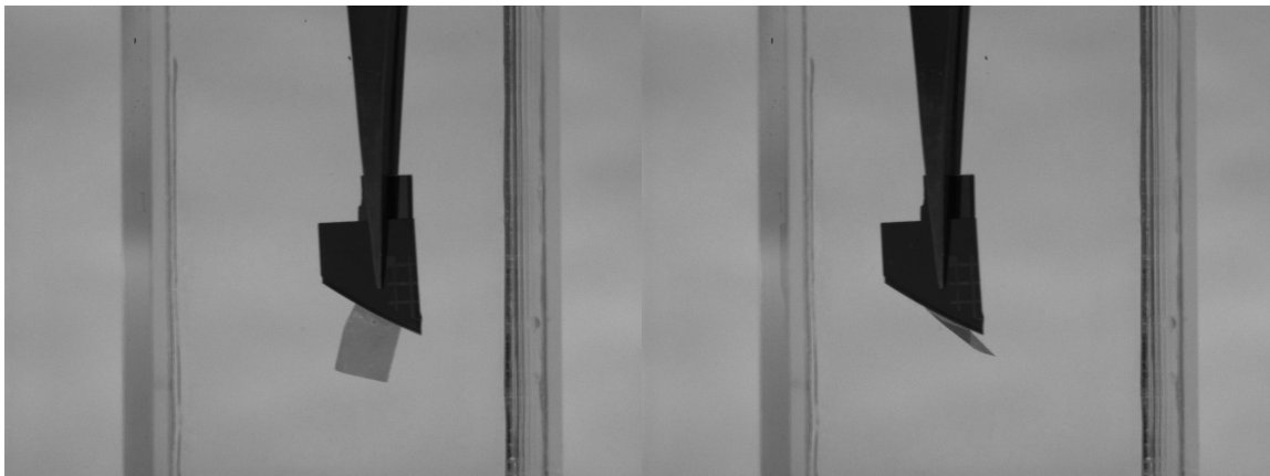
Figure 19: Nanoflag sandwiched between silicon wafer fragments (left). Nanoflag waving as EtOH resists its motion (right).
