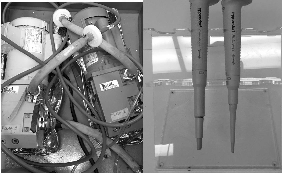
Figure 4: Vacuum Pumps (left). Volumetric Pipettes used to transfer nanofilms, Acetone, and Ethanol (right)
