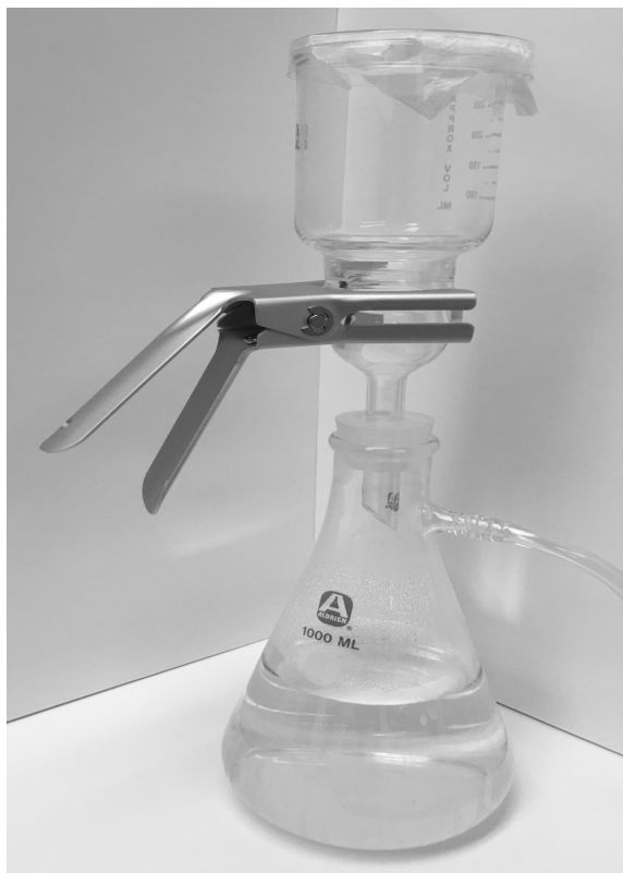
Figure 2: An image of the vacuum film filtration system (VFFS) used to produce the thin films of SWCNTs
