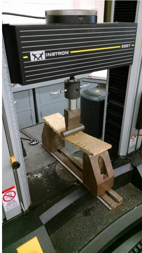
Figure 22. Three Point Static Bending Test
