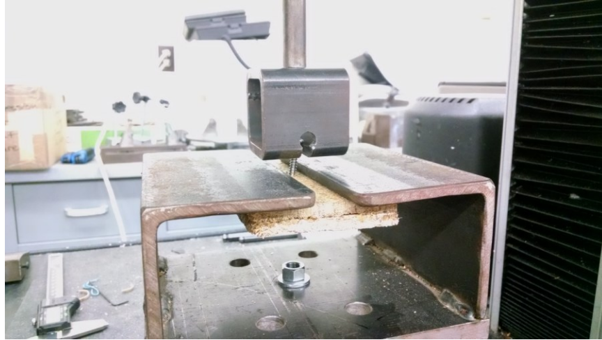
Figure 24. Screw Withdrawal Testing Fixture and Loaded Sample
