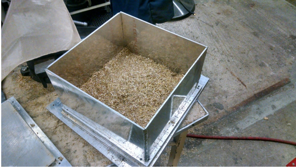
Figure 12. Guide Used to Disperse Fibers Evenly Through Mold
