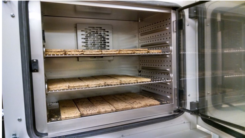
Figure 21. Linear Expansion Samples as Placed into the Conditioning Chamber
