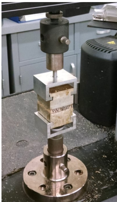
Figure 23. Internal Bond Testing Fixture with Loaded Sample
