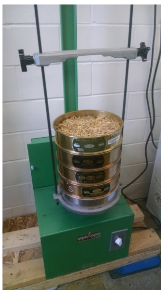
Figure 27. Humboldt H-4325 Series Sieve Shaker with Sieves and Fiber
