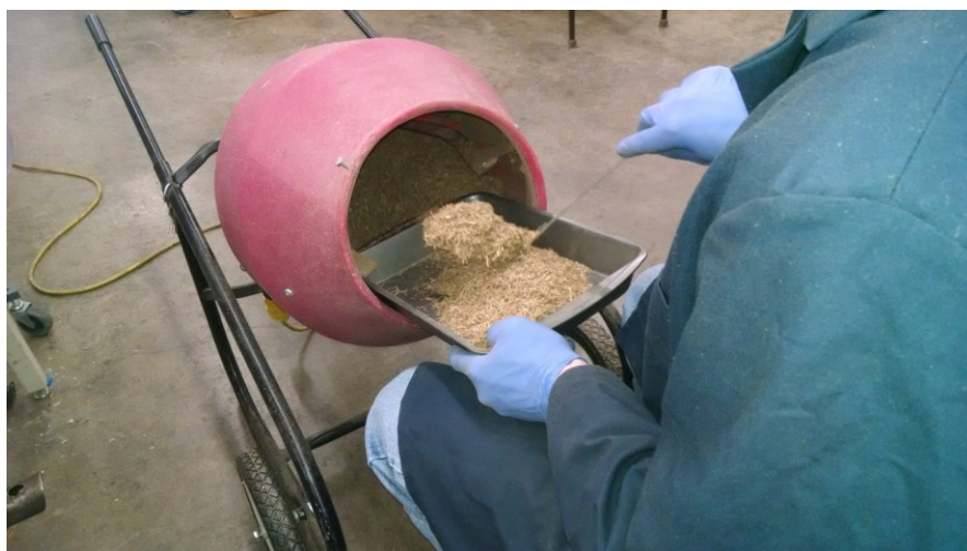
Figure 10. Cement Mixer used to Agitate Fibers During Spraying
