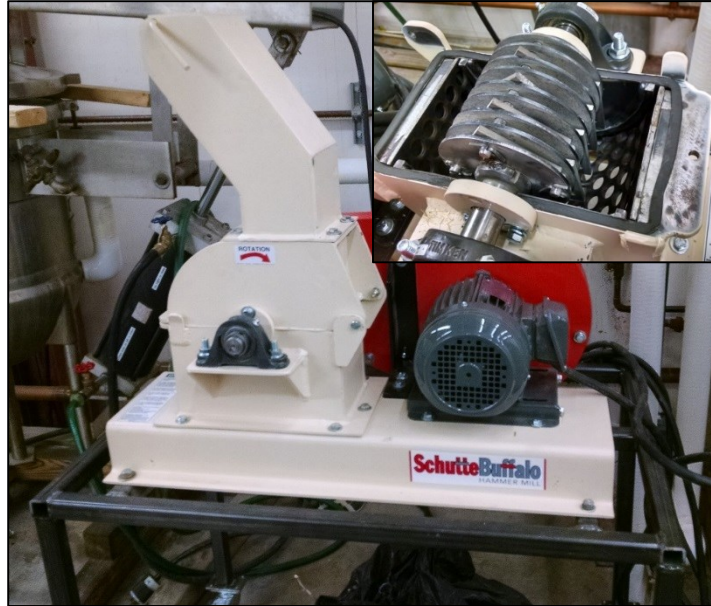
Figure 26. Schutte Buffalo Hammer Mill with Inset Showing Hammers
