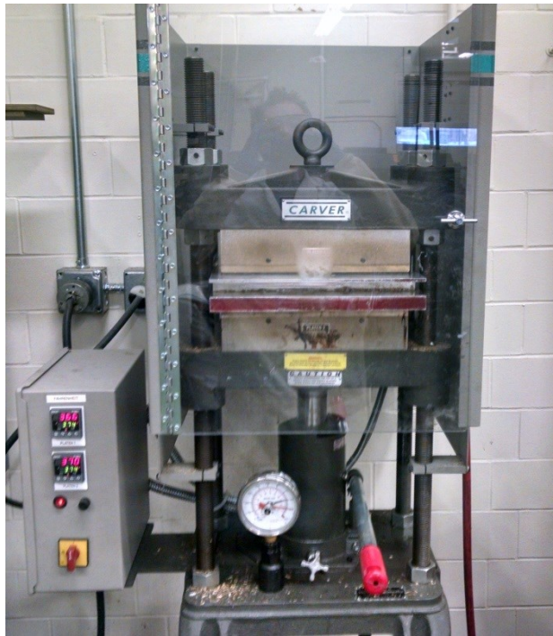
Figure 13. Carver Hot Press with Mold Being Pressed Between the Heated Platens
