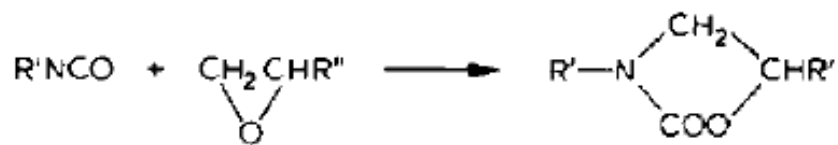
Figure 4. Reaction between Isocyanate (R'NCO) and Epoxide Ring (CH 2 CHR'') to Form an Oxazolidone Ring [34]
