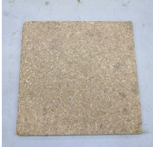
Figure 15. Cooled Board after Being Removed from the Mold
