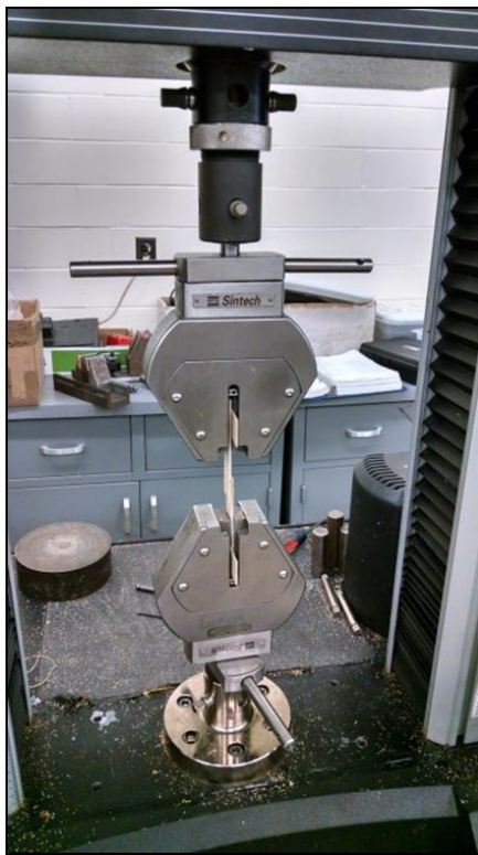
Figure 9. Lap Shear Testing Apparatus and Loaded Sample
