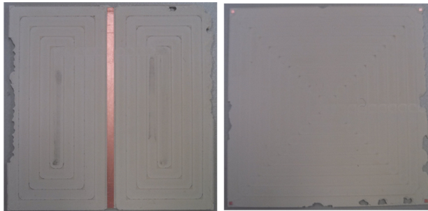
Figure 4.37. Milled top layer for the VEPS with the 50 \Omega trace on the left and the non-cladded back on the right
