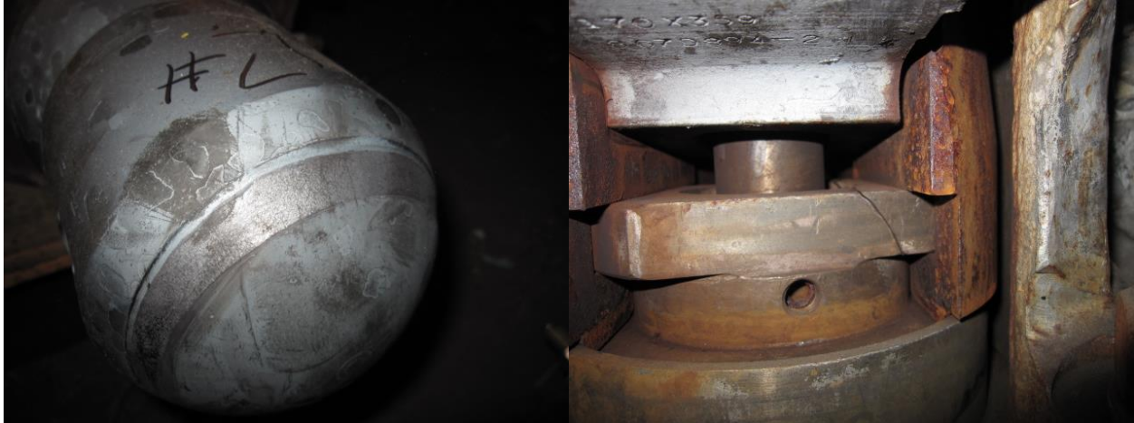
Figure 1.2. Vibration-Induced Damage to Valve 7 [5].
