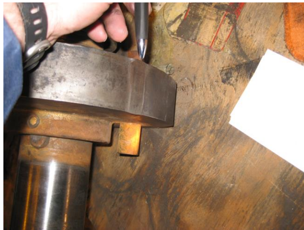
Figure 1.3. Divot in Camshaft Cam due to Valve Vibrations [5].
