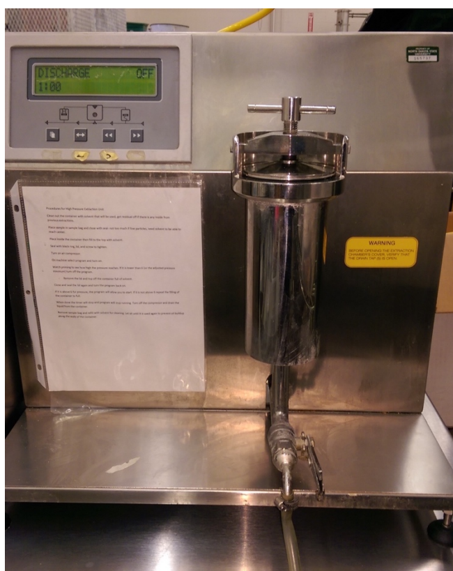
Figure 4. High pressure solvent extraction (HPSE) (Supercritical Fluid Technologies Inc.) unit for flour extractions.
