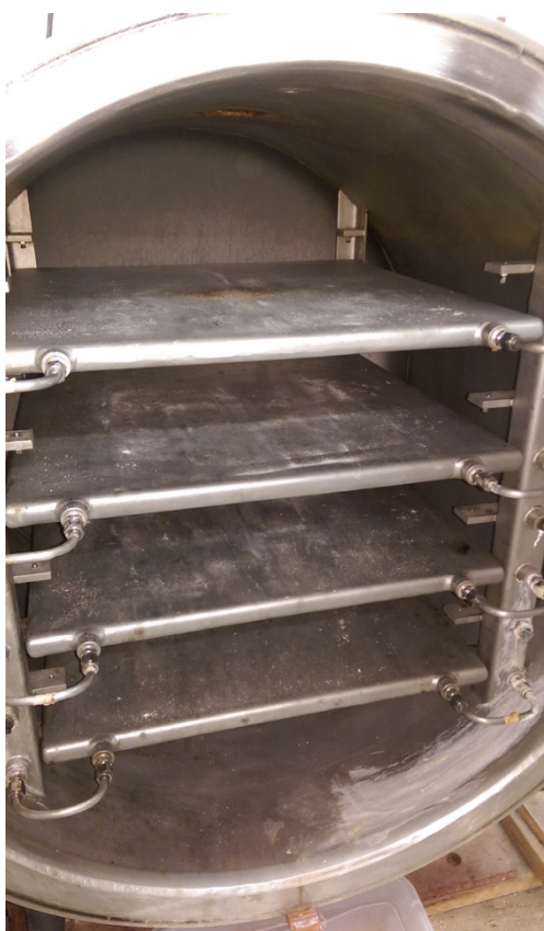
Figure 5. Interior of vacuum oven (Buflovak Buffalo, NY, USA) used for drying treated flours.
