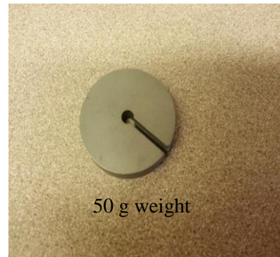
Figure 6. (a) Glutograph (b) Top view (c) Loading weight where the lower the loading weight, the longer the shearing time
