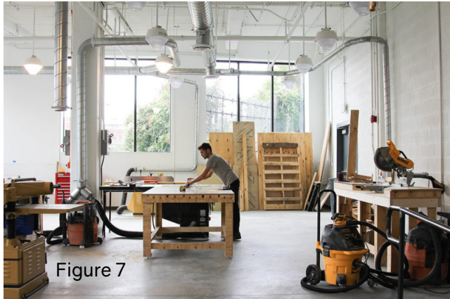
Figure 7 This image shows the relationship between one of my case studies and a section cut of my final project. Note the ceiling heights, exposed structure, and material usage, as well as the large spaces between machines to allow for efficient circulation. A contrast occurs in the method of storage, which can be seen in the southern section cut (below).
