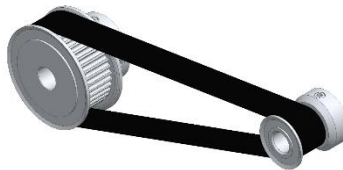
Figure 15. Lead screw belt drive components
