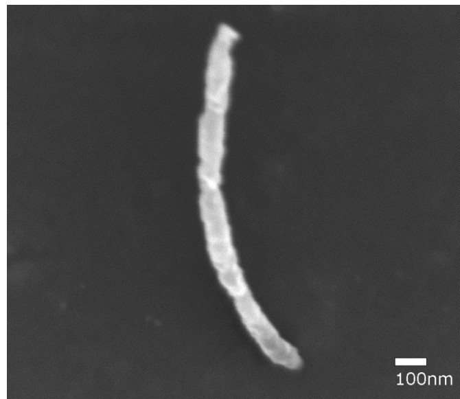
Figure 39. SEM image of a representative MWCNT on the surface of a test specimen.
