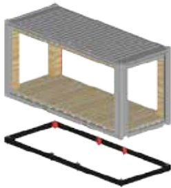
1 - Regular steel frame with eight connections
