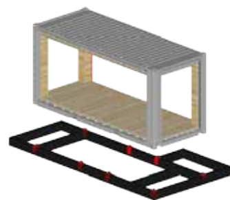
6 - Modified, modular steel frame w/ twelve stationary connections & built to align to final grid
