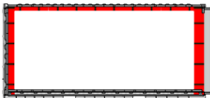
13 - Adding InSoFast continuous insulation panels
