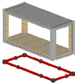
3 - Regular steel frame with four stationary connections and six slidable connections to allow varied configurations
