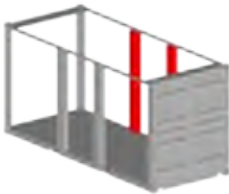
7 - Adding more columns to allow openings on all sides of container
