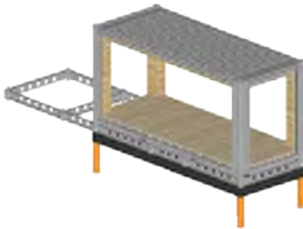
7 - Adding more columns to allow openings on all sides of container
