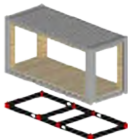
5 - Modified, modular steel frame w/ eight stationary connections & built to align to final grid
