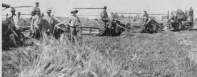
McAndrew Farm about 1911 — Big Four tractor with four independent binders pulled in tandem.
