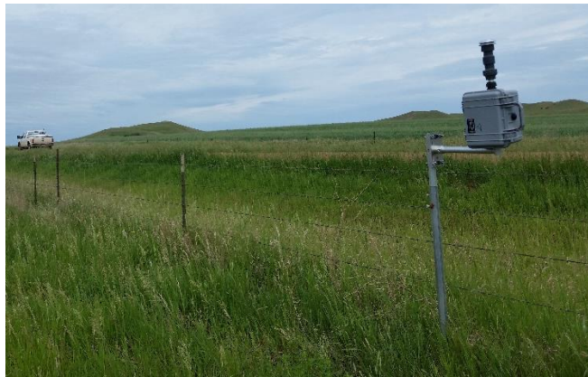
Figure 6. MiniVol™ Portable Air Sampler in operation at site #1 (vertically mounted)
