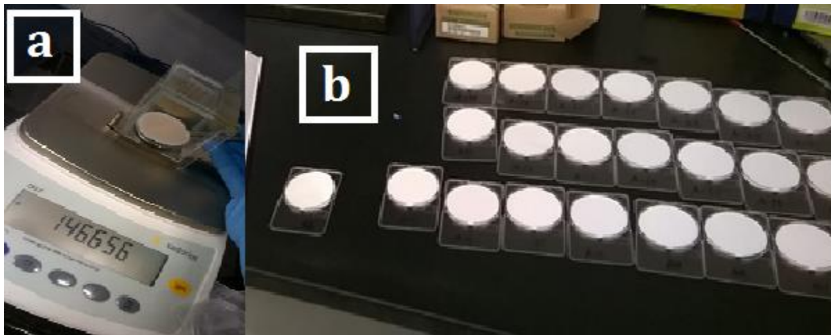
Figure 7. a. Sartorius CP2P Microbalance at CNSE Lab, NDSU; b. Millipore Quartz Filters while being conditioned.
