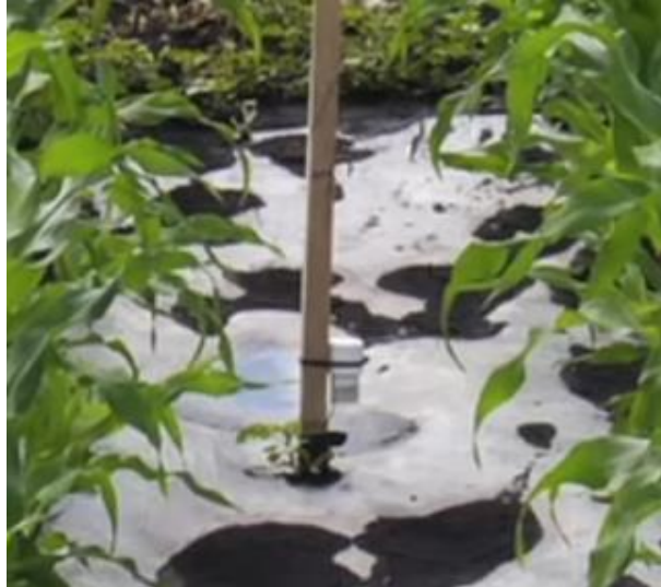
Figure 3: Picture of the air temperature sensor with a radiation shield.
