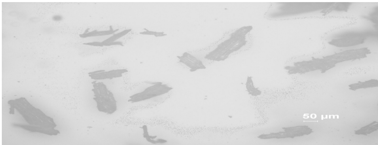
Fig. 5.1: Fibers of WF 30 PLA composite at cycle 0 (magnification 10 X).
