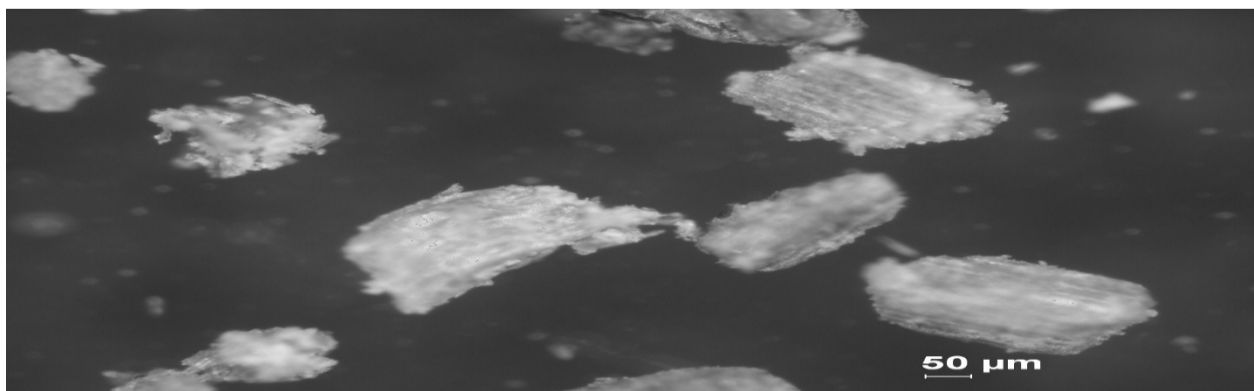
Fig. 4.2: Image of fibers of WF 50 HDPE composite at cycle 6.
