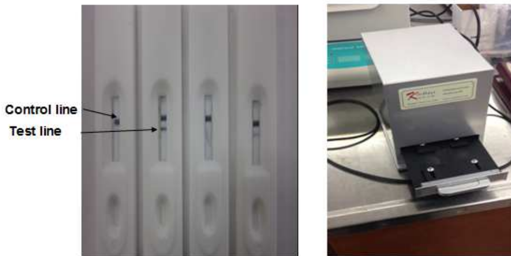
Figure 2.1. Lateral flow strips placed into cuvettes and the color intensity reader: Analyzer DT 1030.
