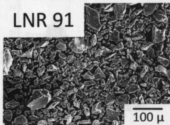
Figure 3-6. Particle shape and morphology of Mg alloy pigments: AM60, AZ91B and LNR91.
