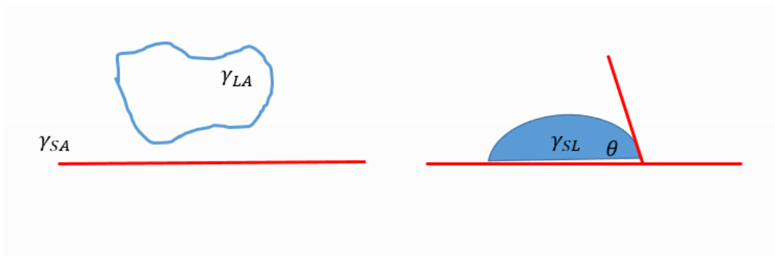
Figure 4.3: Adhesional wetting and contact angle
