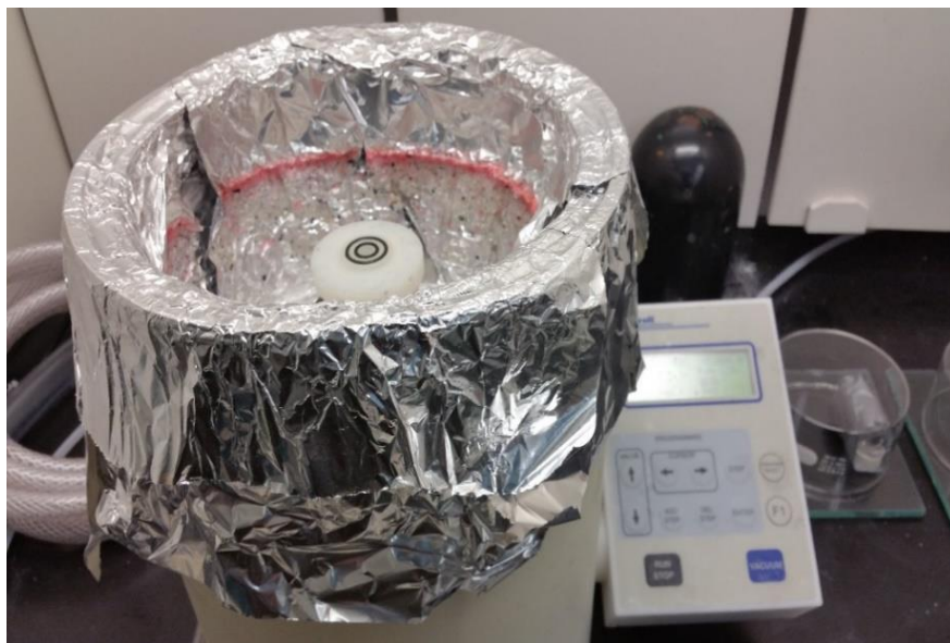
Figure 7. Spin coater was used to produce PS films with nanoscale thickness.
