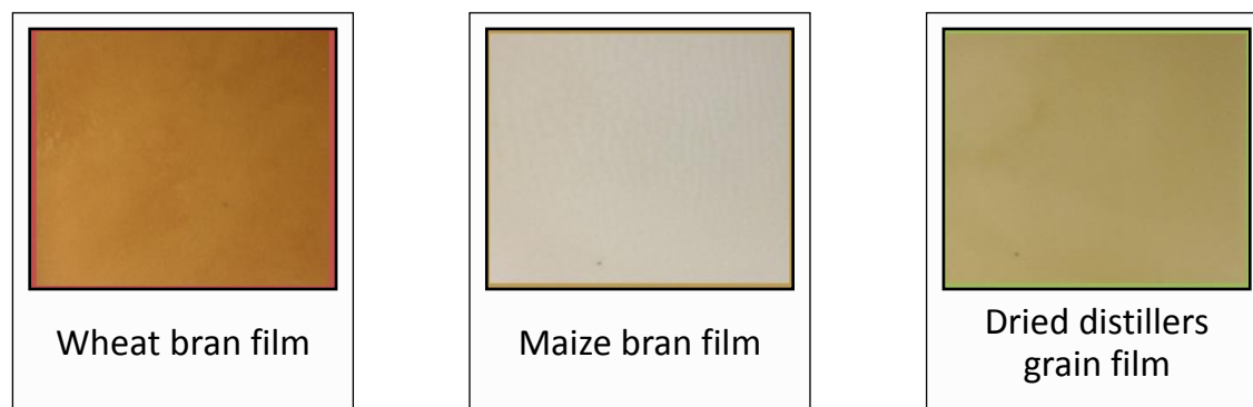
Figure 4.3. Comparison of the colors of arabinoxylan films made using wheat bran arabinoxylan, maize bran arabinoxylan, or dried distillers grain arabinoxylan.
