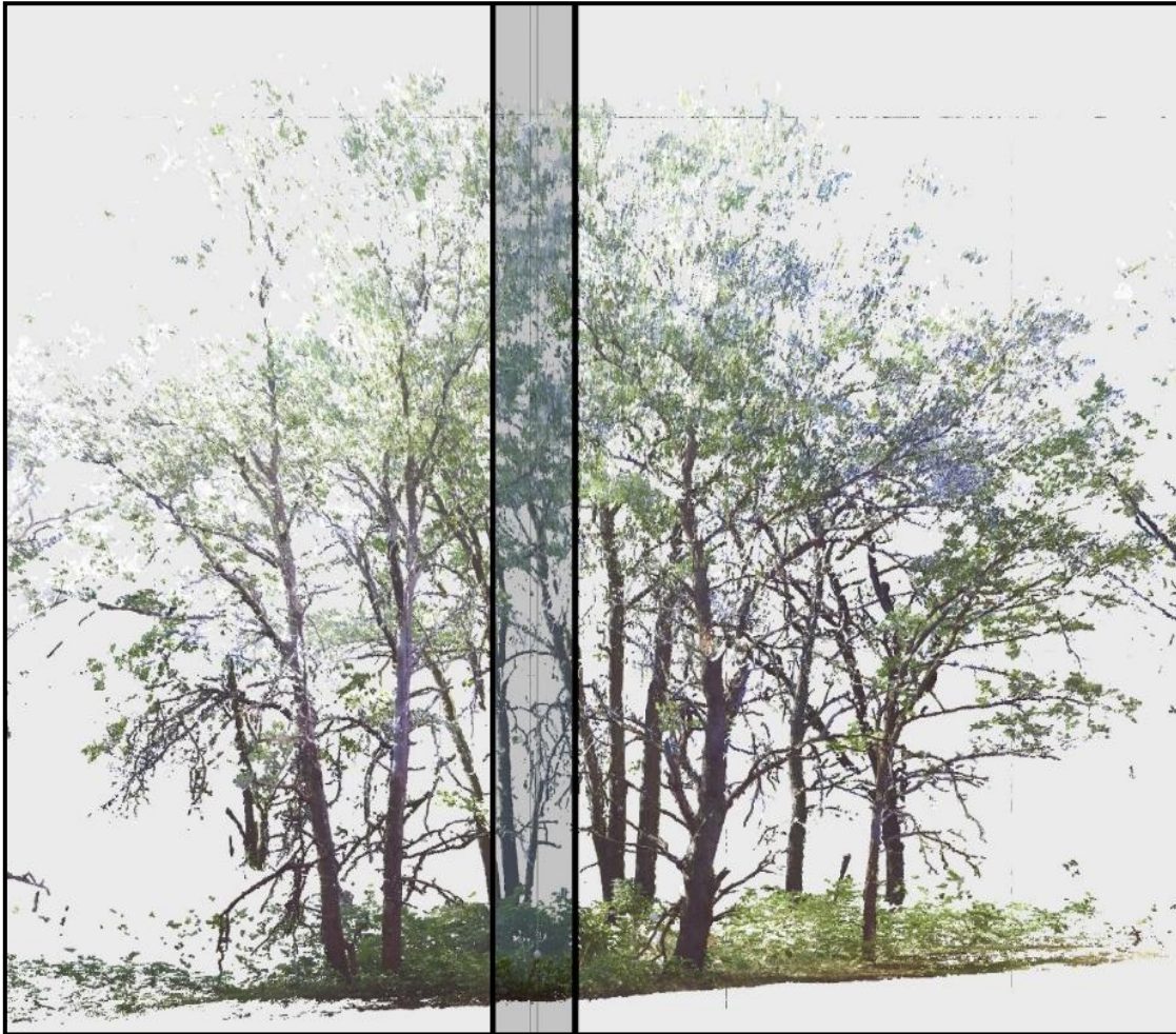
Figure 2.4: TLS scan with area of interest isolated for exportation.
