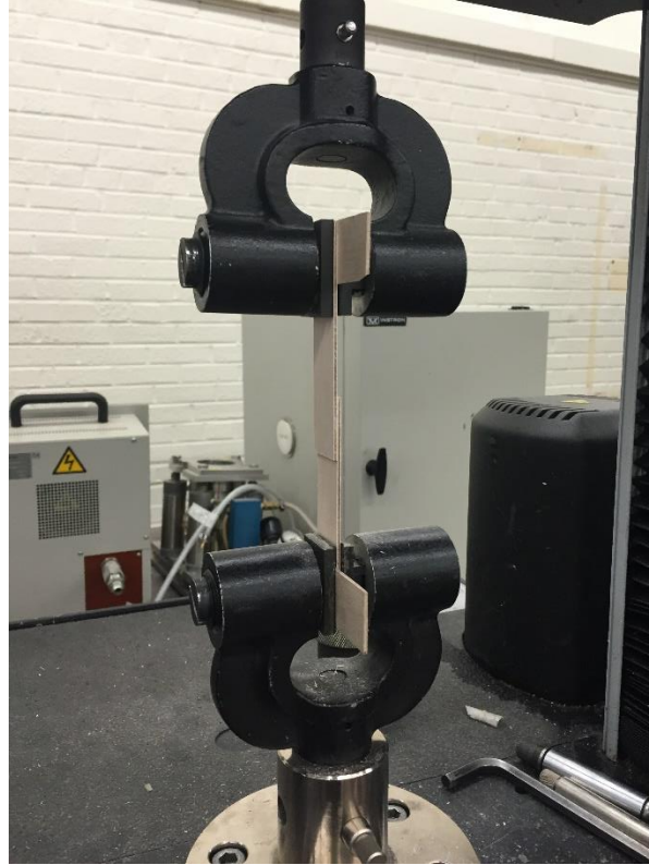
Figure 2-4. Single-lap shear test on Instron 5567.
