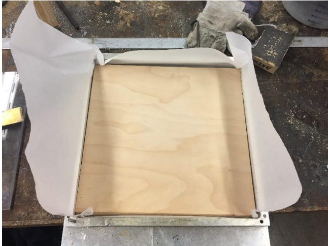
Figure 2-6. Photo showing three layers of birch sheets stacked in an aluminum mold before pressing.
