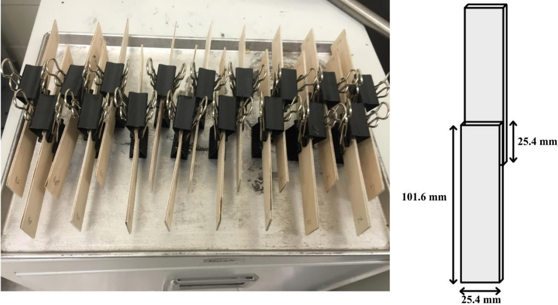
Figure 2-3. Preparation of the single-lap shear test samples and the dimensions of the samples.
