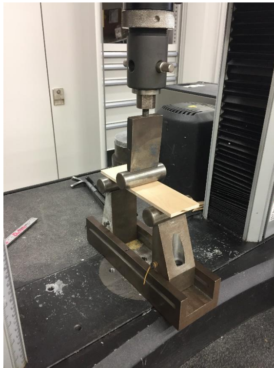
Figure 2-8. Three-point bending test of plywood specimen.
