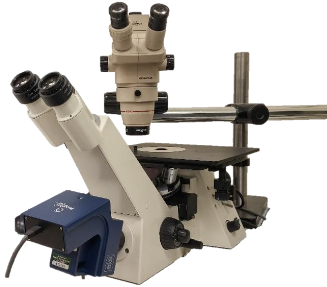
Figure 4.6: Zeiss microscope and JENOPTIK camera used to measure bond line thicknesses
