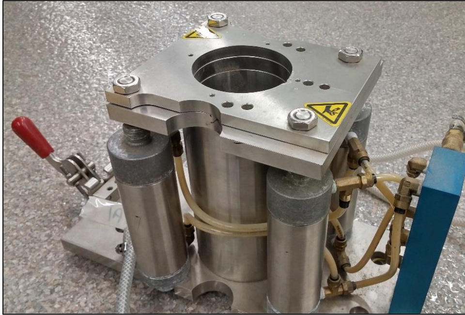
Figure 4.17: Pneumatic clamping mechanism used to secure impact specimens
