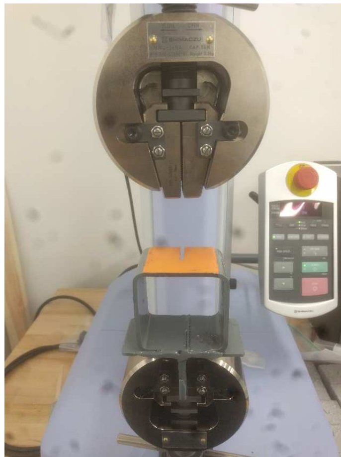
Figure 12. Steel fixture mounted into Shimadzu
