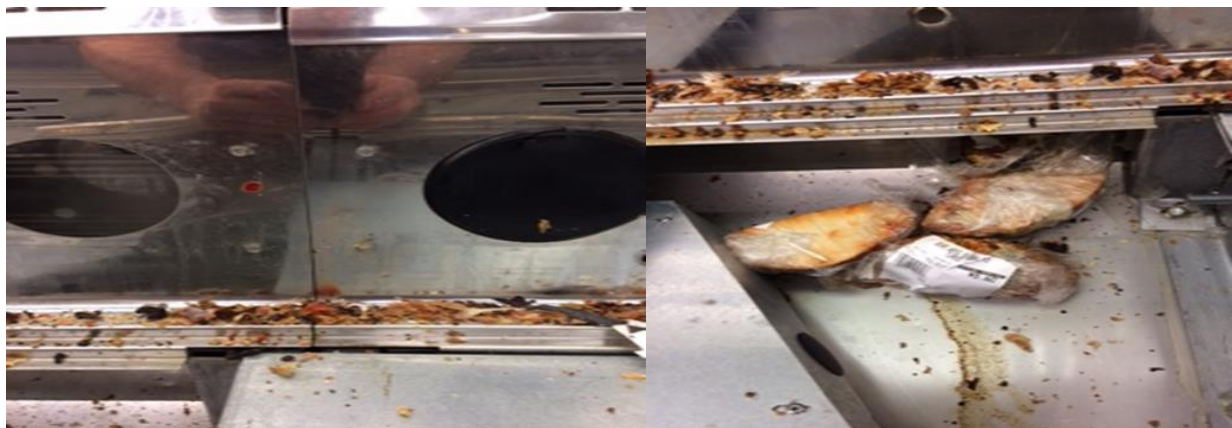
Figure 1. a) Interior of deli display case with vent covers missing. b) Interior of deli display case with 4-month old deli meat.
