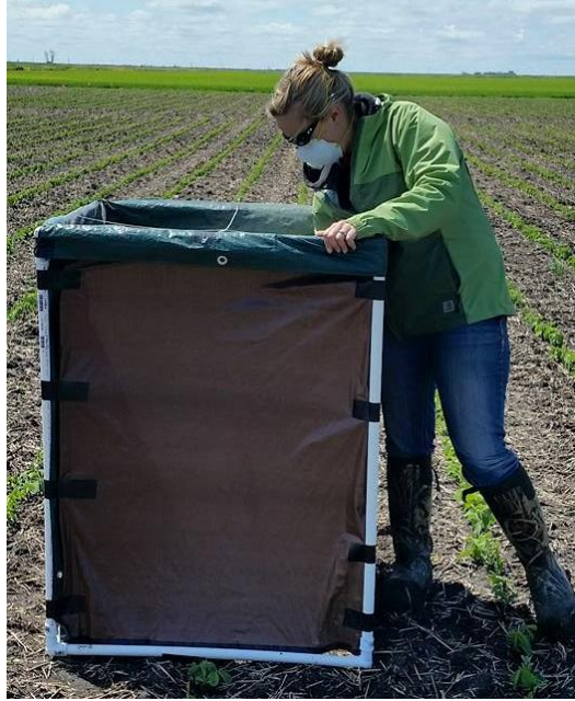
Figure 2.3. Dust spray booth during dust application.
