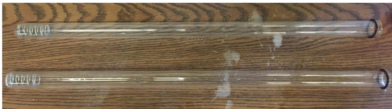
Figure 4.9. Visual comparison between fouled and clean quartz sleeve at the end of C15.
