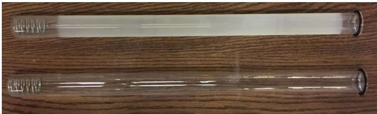
Figure 4.6. Visual comparison between fouled and clean quartz sleeve at the end of C14.
