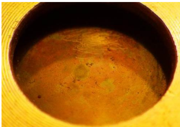
Figure 4.2. Magnified picture of the fouled UV intensity sensor.
