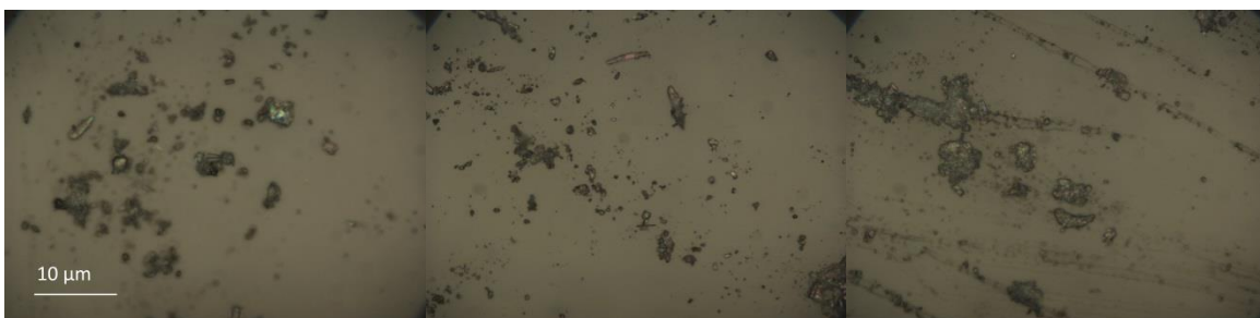
Figure 49. PS-PAA-PS 1:50:1 passed through excess toluene in separatory funnel at 50x magnification.
