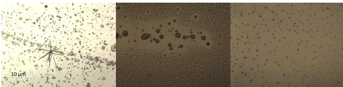
Figure 41. PS-PAA-PS 1:50:1 added dropwise to ~20mL of toluene at 50x magnification.
