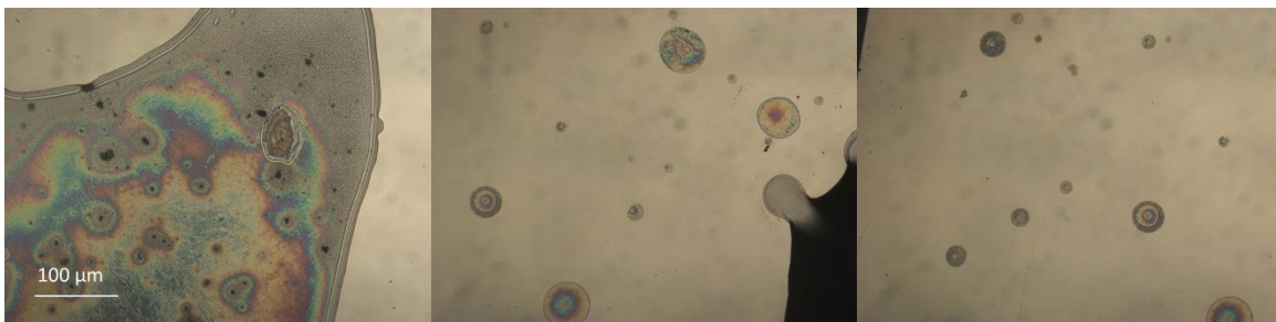
Figure 46: PS-PAA-PS 1:20:1 mixed in toluene for 24 hours at 5x magnification.
