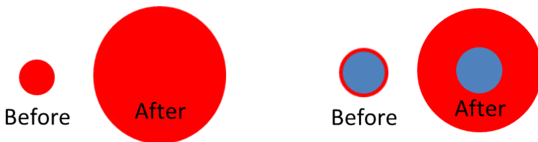
Figure 25. A general schematic of particle swelling. Before indicates a particle in an unswelled state and after indicates a solvent swollen particle. The left pair shows a standard microgel particle. Swelling of phase separated amphiphilic block copolymer particle is shown in the right pair of images. Blue is the core block and red is the outer solvent responsive block which collapses in bad solvents, before, and swells in good solvents, after.
