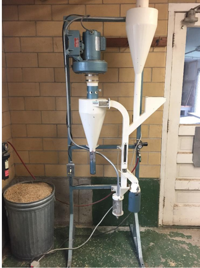
Figure 6: Codema Laboratory Oat Dehuller
