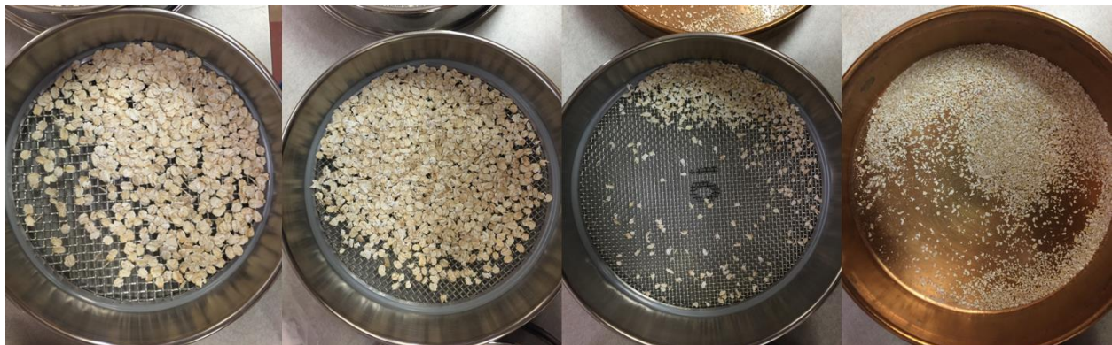
Figure 11: Sample Remaining on Ro-Tap Sieves From left: US standard sieves # 4, 7, and 10, bottom pan.
