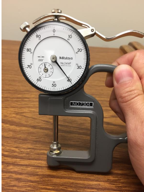
Figure 9: Thickness Gauge with Oat Flake
