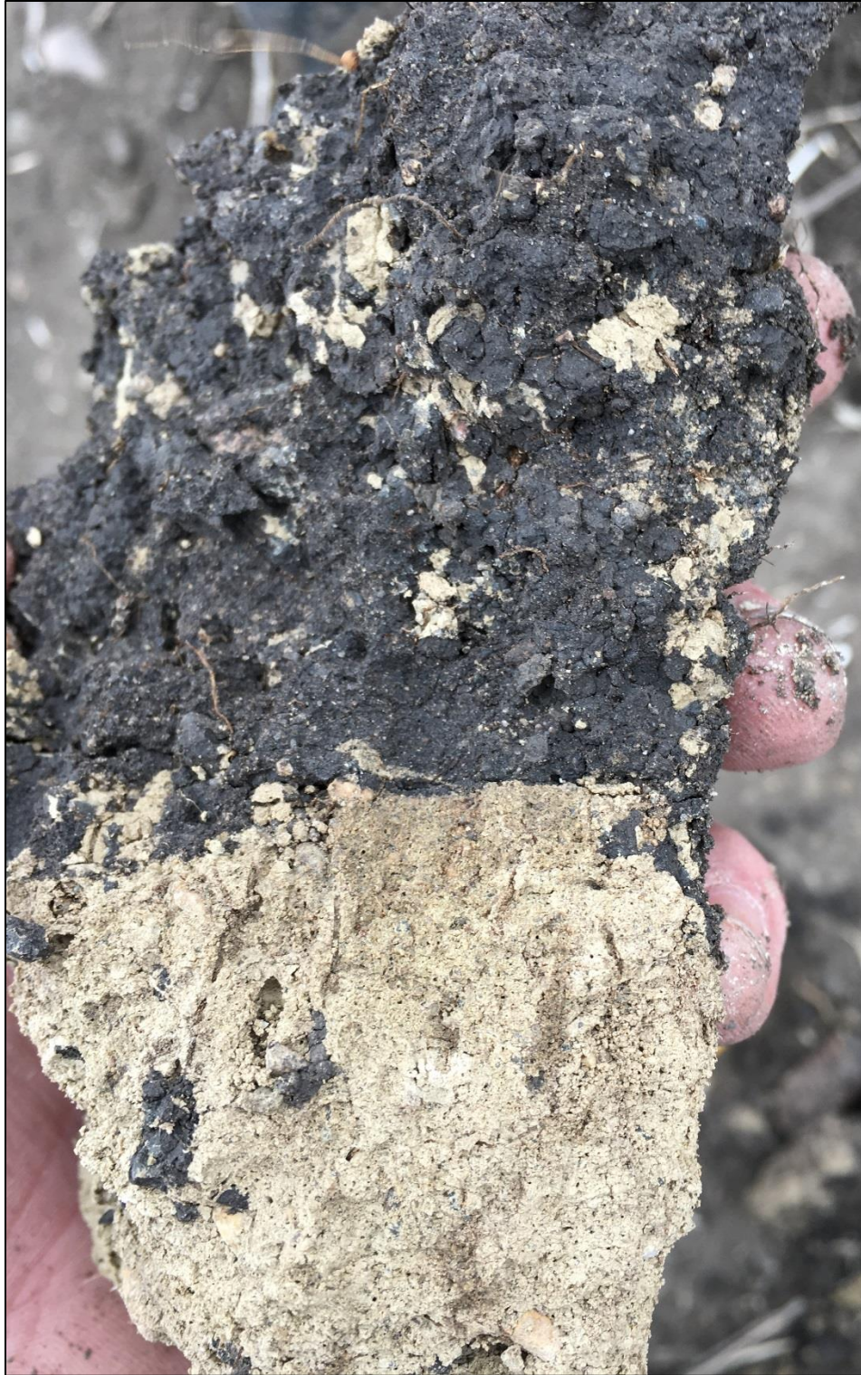
Figure 24. A very abrupt boundary between the mollic epipedon (top) and the calcic horizon (bottom). Note the remnant light brown cambic material truncated and mixed into the profile. Cambic colored earthworm casts are also noticeable in the top horizon (2A10).
