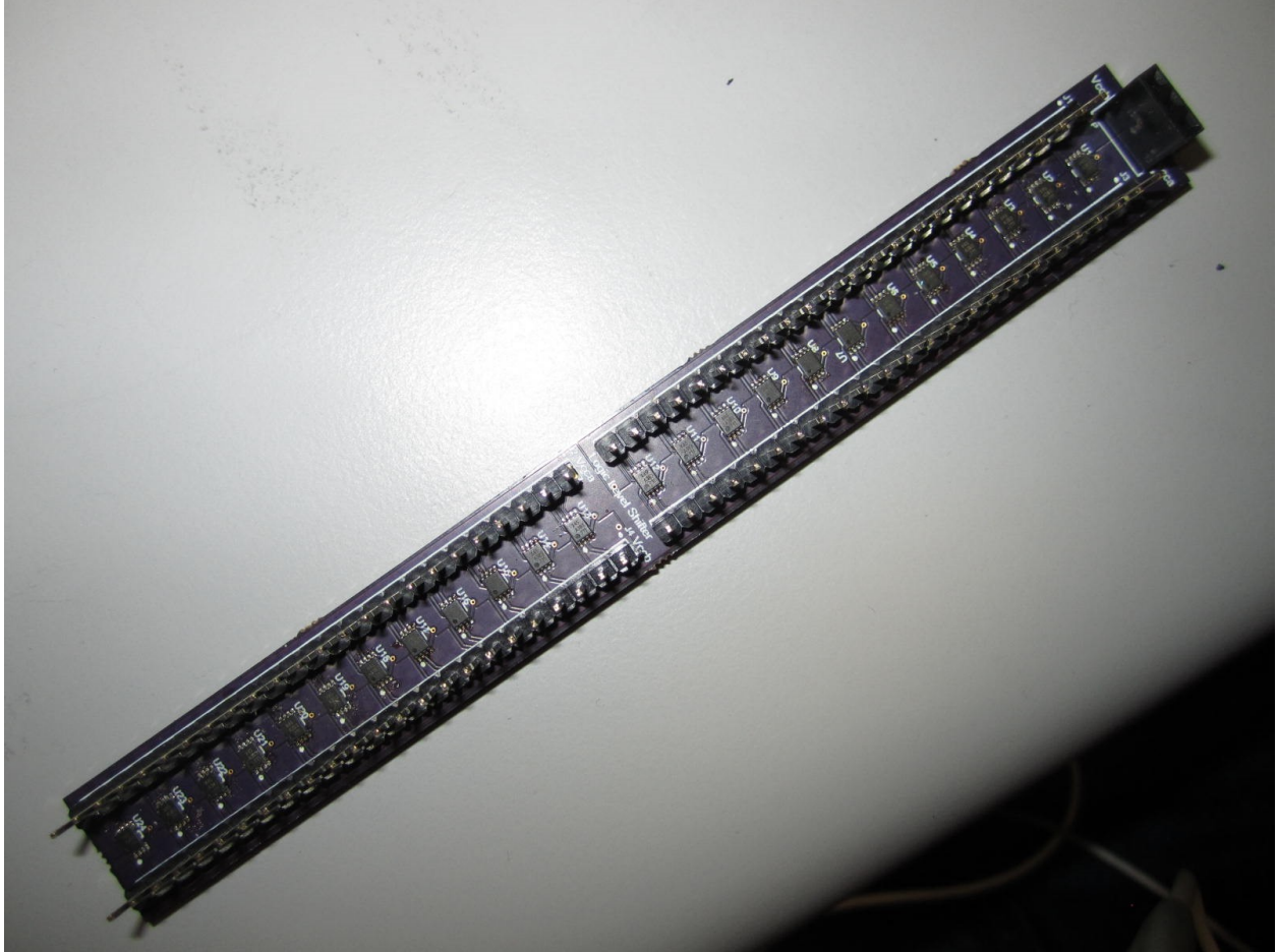
Figure A.5. Front side of the level shifter PCB.
