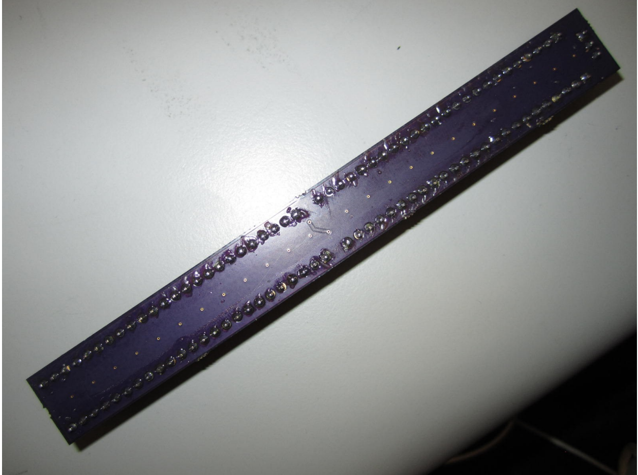
Figure A.6. Reverse side of the level shifter PCB.
