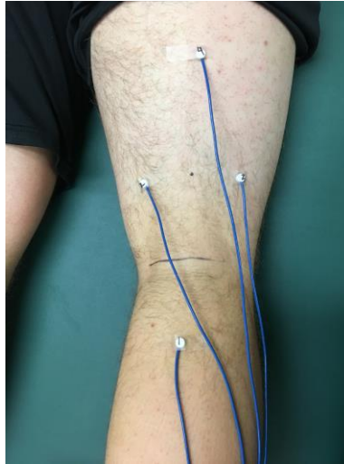
Figure 3. Application of thermocouples for measuring skin temperatures.
