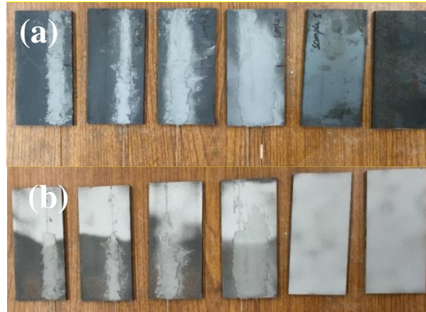
Figure 4.4. Prepared samples (a) after sensor embodiments and (b) after sand blasting.
