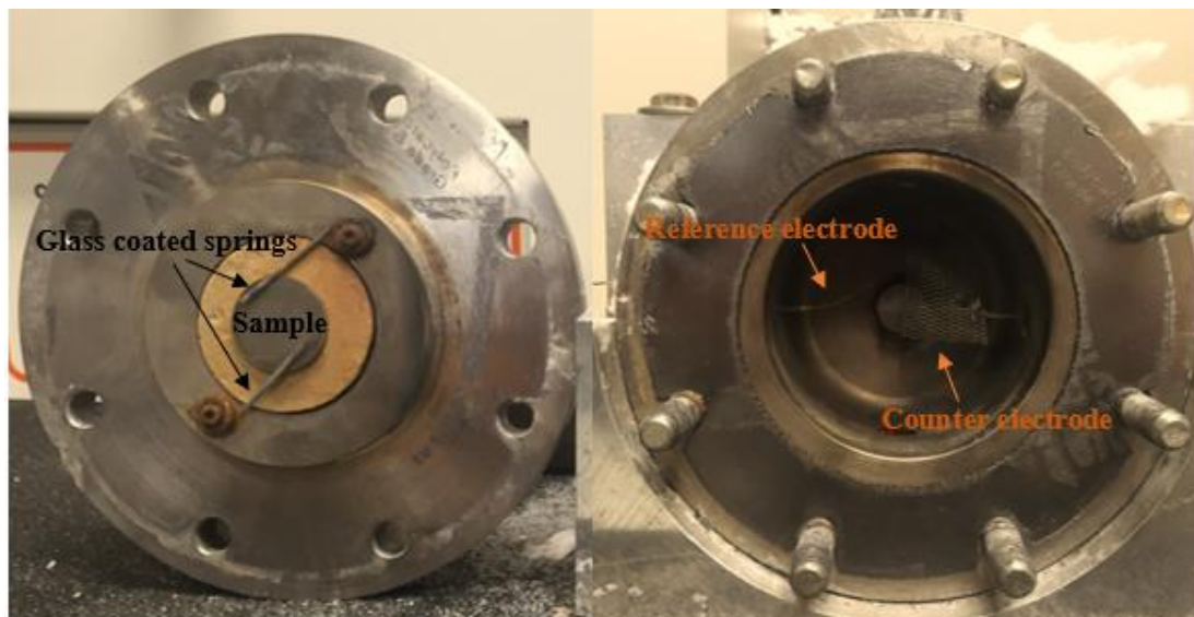
Figure 4.9. Sample and electrode placement inside the pressure vessel.
