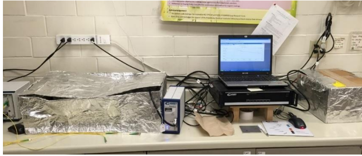
Figure 4.7. Electrochemical Accelerated Corrosion Tests Equipment Set-up.
