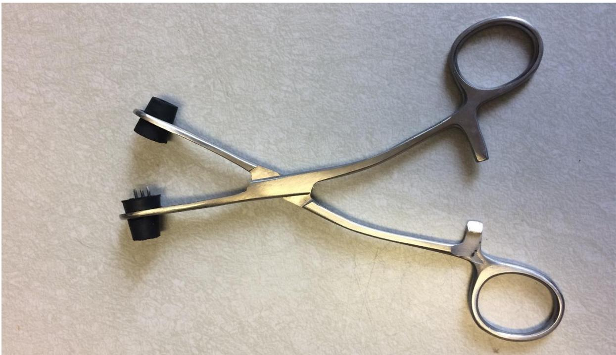
**Figure 2.2.** Three pins fitted in a line across rubber stopper inserted into tongue-seizing forceps. Pins serve to wound corn leaves at the point of inoculation.
