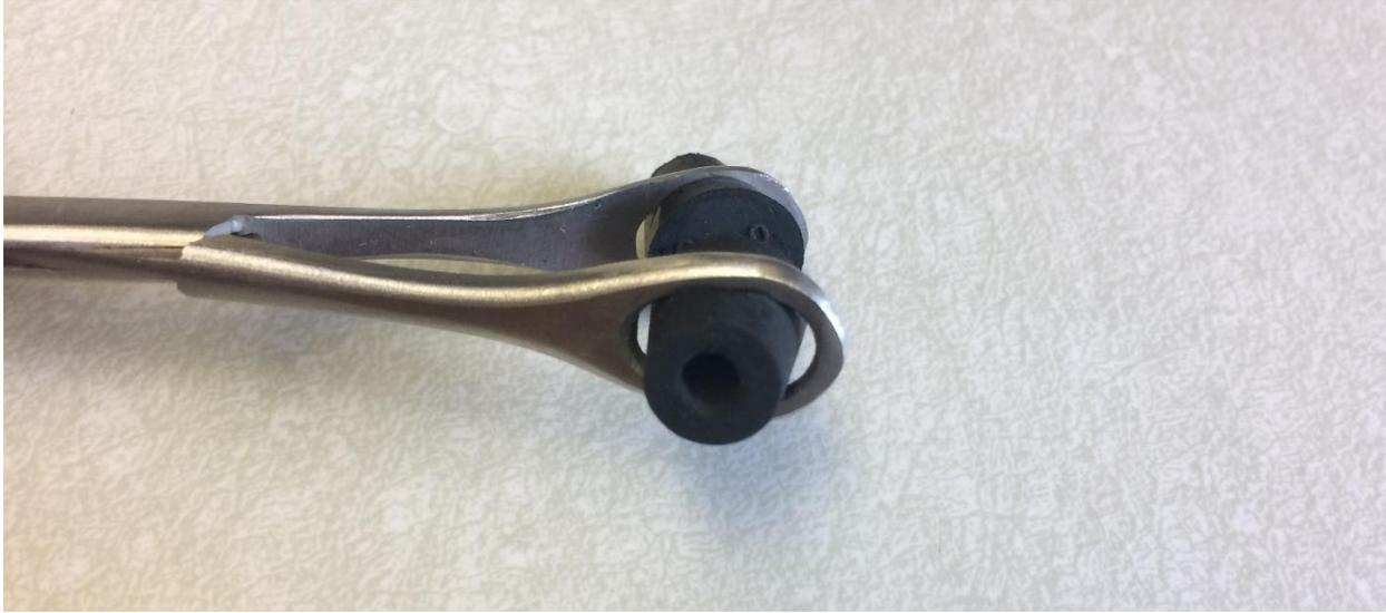
**Figure 2.3.** Gauged rubber stopper inserted into tongue-seizing forceps. A 1 ml syringe is fitted into the stopper to deliver *Clavibacter nebraskensis* inoculum into wounded corn leaves.
