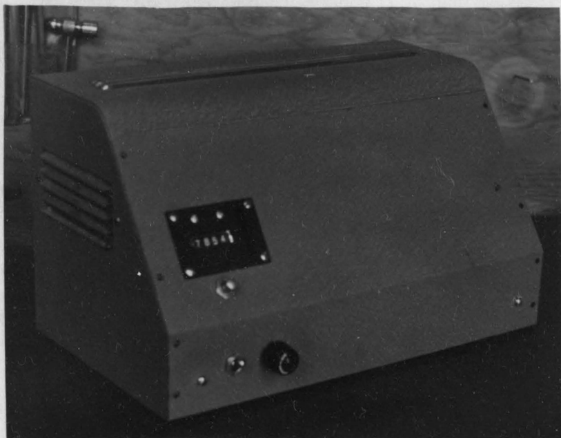
Figure 22. The Slip Frequency Detector Mounted in Cabinet.
